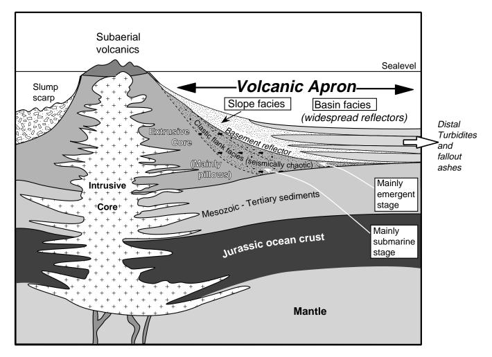
Figure 7. Schematic drawing of an ocean island and its clastic volcanic apron. The intrusive and extrusive core facies is overlain by the seismically "opaque" flank facies consisting of basaltic volcaniclastic rocks of the submarine and emergent stage. The sediments of the volcanic apron above the basement reflector are subdivided into a slope facies characterized by slumps and the basin facies with more continuous reflectors. Modified from Schmincke (1994).
