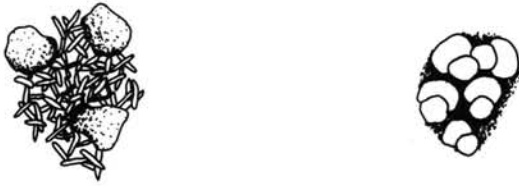
(a) Matrix-supported aragonite Interparticle porosity: high Intraparticle porosity: low Total porosity: medium Permeability: medium (b) Matrix-supported (clay and smaller particles) Interparticle porosity: low-medium Intraparticle porosity: high Total porosity: medium-high Permeability: low-medium
