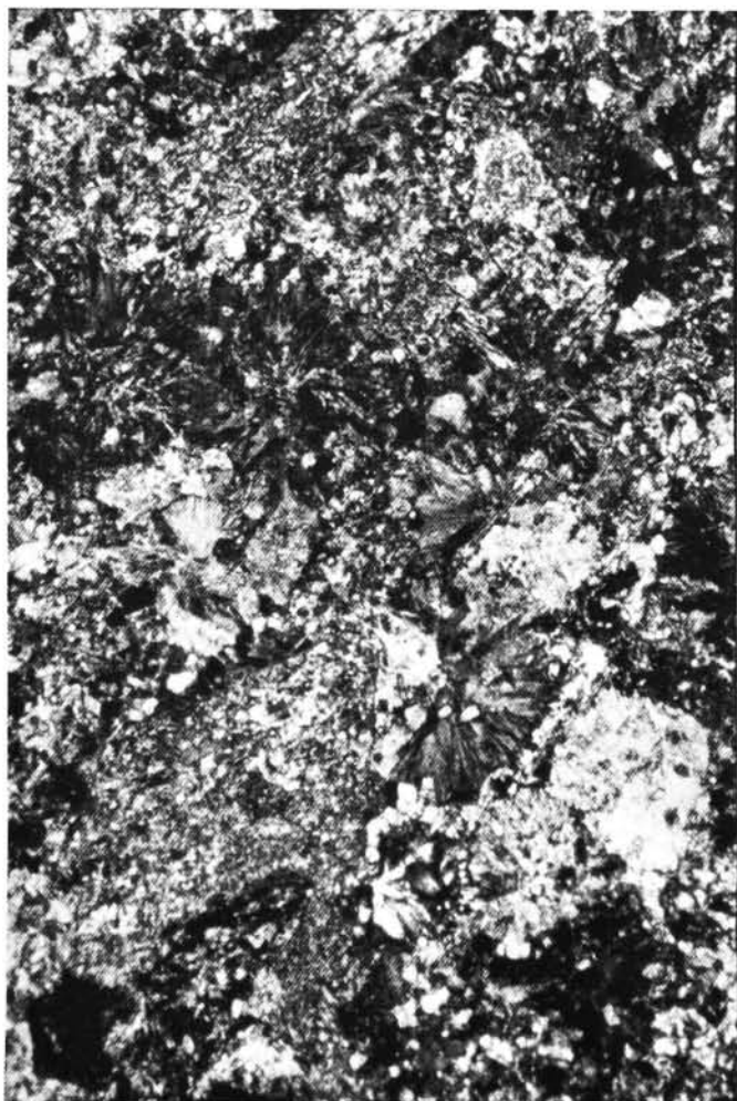
Figure 15. Photomicrographs of representative features in groundmass of rhyolitic rocks from Hole 639F. A. Sample 103-639F-2R, CC, 18–20 cm. Altered feldspar phenocryst (right center) surrounded by radiating groundmass material. Field of view is 3.6 \times 2.4 mm. B. Sample 103-639F-2R, CC, 9–11 cm. Altered feldspar phenocryst surrounded by radiating structures in the groundmass. Field of view is 3.6 \times 2.4 mm.
