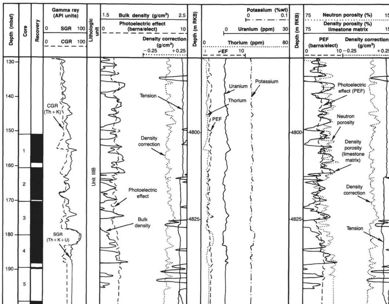
Figure 21. Composite log and core recovery, Hole 641C. See text for description of logs.
