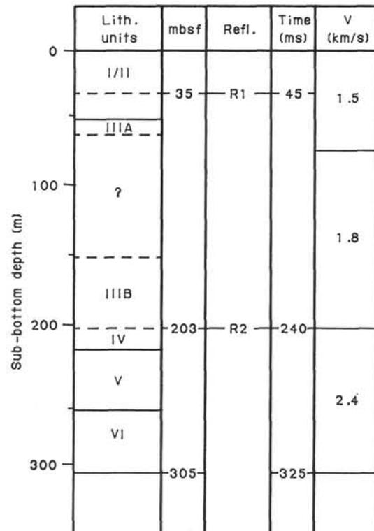
Figure 24. Correlation between lithologic units (see "Sediment Lithology," this chapter) and reflectors R1 and R2, according to the velocities measured on board (see "Physical Properties" section, this chapter).
