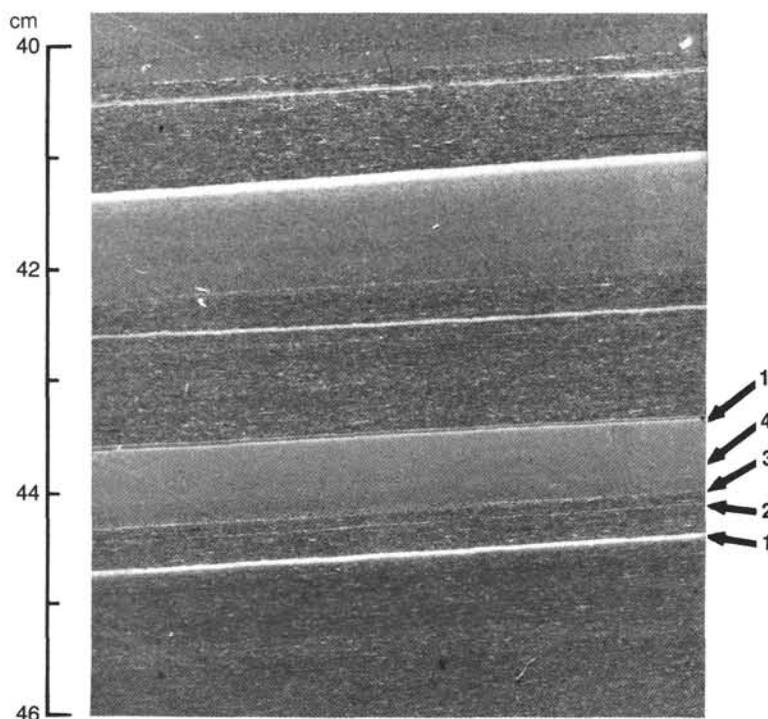
Figure 7. Sample 103-641C-11R-1, 40–46 cm. Typical microturbidites of lithologic Units V and VI. Silty calcareous clay grades upward to massive claystone, which is capped by a thin, light-colored marl lamina. 1, white marlstone lamina at top of microturbidite; 2, laminated silty claystone interval; 3, quartz silt lamina; 4, homogeneous claystone interval.
