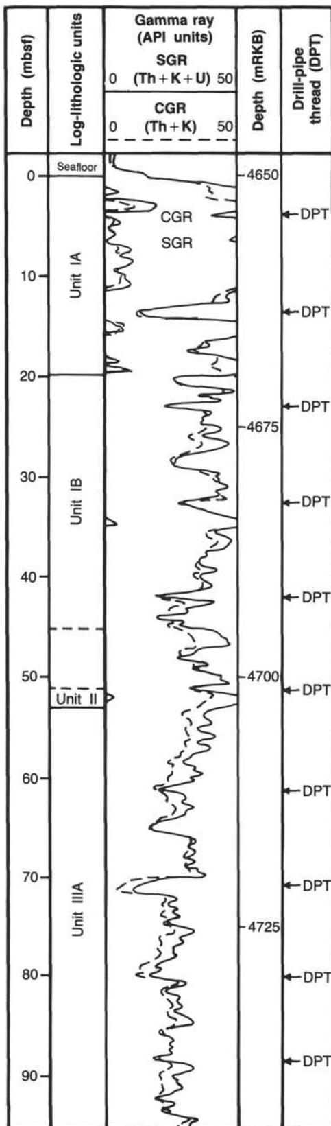
Figure 22. Preliminary correlation of gamma-ray spectrometry log, recorded through the drill pipe in Hole 641C, and lithologic units at Hole 641A. Boundaries of lithologic units are based on logging results and roughly correlate with lithologic units described from the recovered cores (see Table 2).
