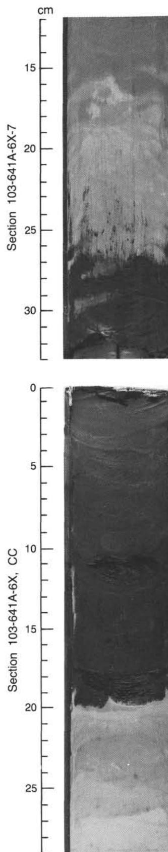
Figure 4. Black zeolitic clay of Unit II (Sample 103-641A-6X-7, 27 cm, through 103-641A-6X, CC, 20 cm), in contact with overlying gray and brown clay of Unit I and underlying greenish gray marl of Subunit IIIA.
