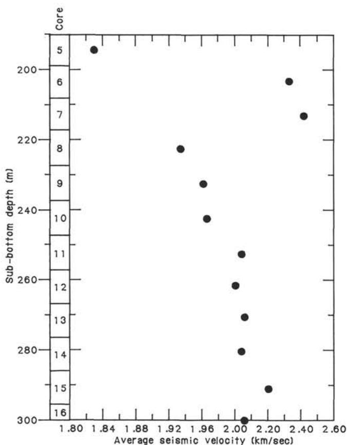
Figure 19. Average seismic velocity of Cores 103-641C-5R through 103-641C-16R plotted against sub-bottom depth (see text for discussion).
