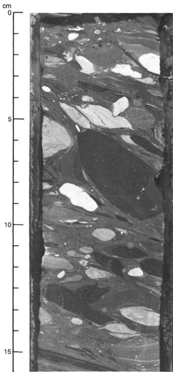
Figure 8. Sample 103-641C-15R-3, 0–17 cm. Typical debris-flow deposit in lithologic Unit VI.
