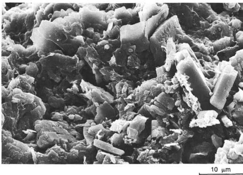
Figure 5. SEM photograph of the black zeolitic clay of lithologic Unit II (Sample 103-641A-6X, CC, 0–3 cm). The sediment is composed almost exclusively of zeolites (altered radiolarians) and clay minerals.
