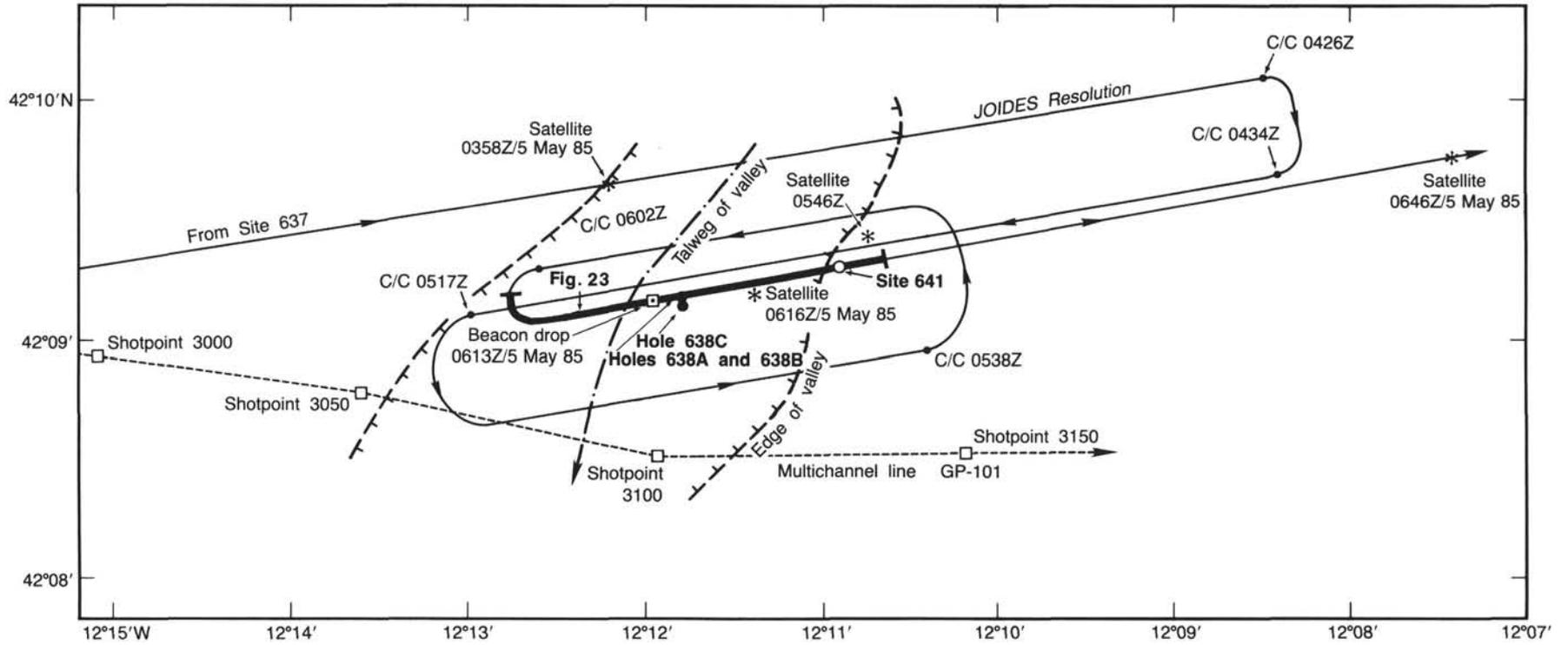
Figure 3. Chart showing the location of Site 641 and its relation to Site 638 and to the track of *JOIDES Resolution* along which a seismic profile was made. Location of IFP seismic line GP-101 is shown by dashed line. Location of *JOIDES Resolution* seismic profile shown in Figure 23 indicated by heavy solid line. Edge of valley, as delineated on *JOIDES Resolution* and IFP seismic lines, is indicated by hachured dashed line.
