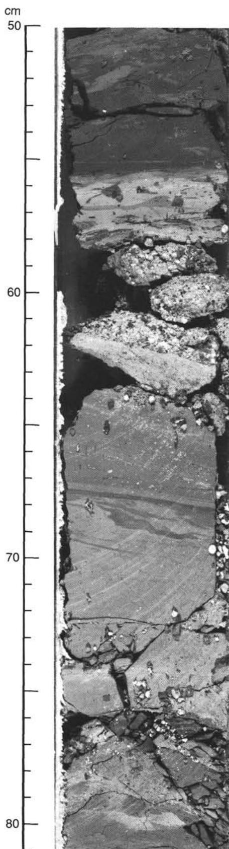
Figure 6. Sample 103-641C-6R-3, 50–81 cm. Contact between lithologic Subunit IIIB and lithologic Unit IV is placed at the top of the uppermost carbonate granule conglomerate at Sample 103-641C-6R-3, 58 cm.
