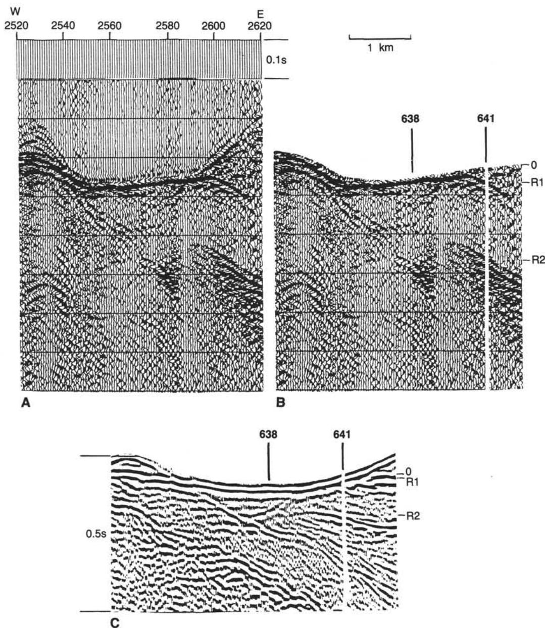
Figure 23. A. Seismic line recorded aboard *JOIDES Resolution*, when surveying the Sites 638 and 641 area. Location of line shown in Fig. 3. B. The same line, with side echos erased, showing the location of Sites 638 and 641. R1 and R2 are reflectors discussed in the text. C. IFP processed seismic line GP-101, onto which Sites 638 and 641 are projected. Location of line shown in Figure 3. Courtesy of L. Montadert.
