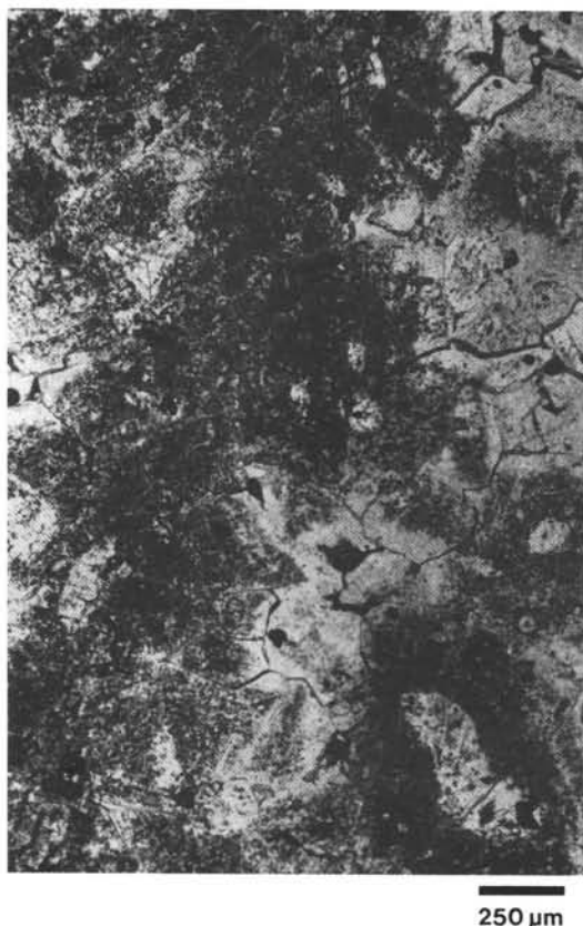
Figure 13. Dirty dolomite texture type 1a. Hypidiotopic texture of subhedral dirty crystals is dominant but is always associated with another textural area composed of clearer, baroque crystals (see text). The contrast between the two textures outlines the original grains. Sample 103-639A-10R-1, 143–144 cm; natural light.
