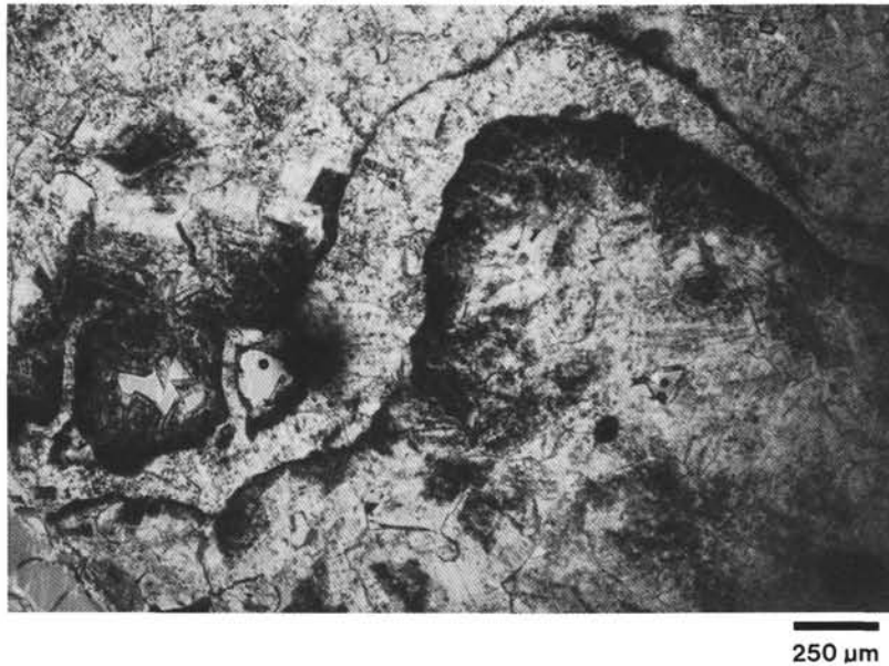
Figure 18. Fissure type F(a) in the dolomite unit is a phantom of an earlier meandering fissure, outlined by the concentration of impurities along the wall. Sample 103-639A-10R-2, 108-112 cm; natural light.
