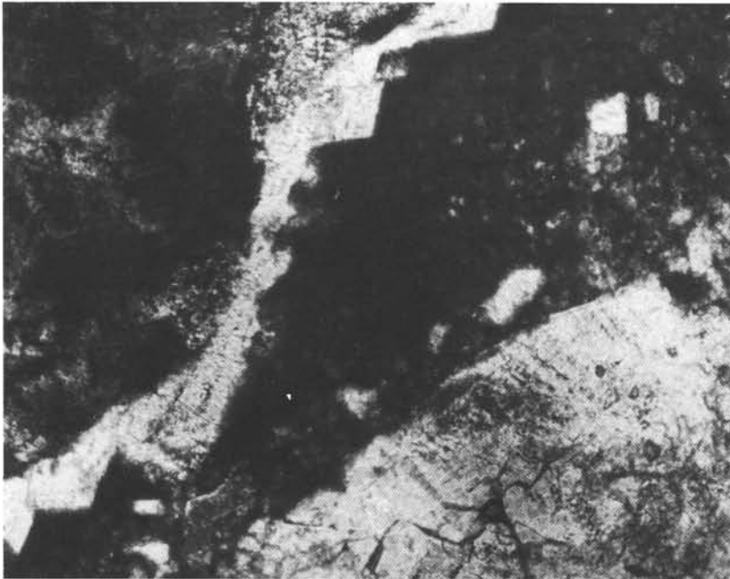
Plate 8. Detrital dolomite filling fissures and vugs. 1. Cathodoluminescence. 2. Natural light. Graded bedding, heterometric microbreccia filling a fracture in dolomite. 1 = host rock with a relatively clear cathodoluminescence corresponding to dirty texture; 2 = fringe of clean saddle dolomite exhibiting a dark cathodoluminescence along the roof of the fissure; 3 = internal sediment composed of a dark matrix (with a very dark to black cathodoluminescence) embedding clean crystalline and lithic debris (with a dark cathodoluminescence); 4 = large dolomite element of the internal breccia showing a truncated and eroded surface. The margin of saddle dolomite and all the sedimented crystals present a final thin black zonation under cathodoluminescence (arrows). Sample 103-639A-10R-1, 81-83 cm. 3. Negative print of a thin section showing a laminated deposit partially coating the surface of a piece of dolomite. This coating appears to be an incompletely recovered filling of a large fissure. The boundary between the host rock and cavity intersects all recognized crystalline textures and is fringed by a transparent (black on negative) rim of baroque dolomite. The laminated sediment was affected by internal gliding planes and resedimentation, which evidence rapid lithification. Sample 103-639A-10R-1, 40-44 cm.
