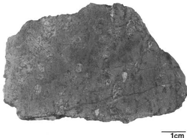
Figure 3. Sample 109-670A-6R-1 (1-10 cm). The top of the sample is at the left. The subhorizontal trace of the foliation is marked by elongated orthopyroxene and spinel grains.
