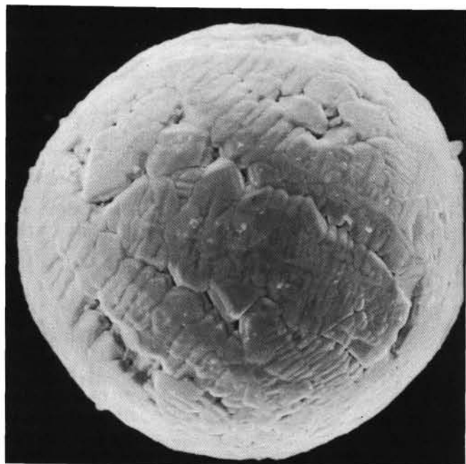
Figure 22. SEM photo of black sphere (approximately 0.2 mm diameter), tentatively identified as a micrometeorite. Sample is from 107-652A-28R, CC.
