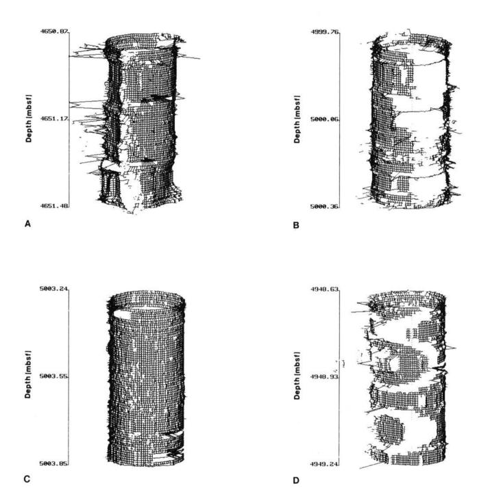
Borehole televiewer images from Hole 504B; information on stress and structure. A. Clean, well-defined breakouts. B. Major breakouts with no reflected signal. C. Competent rock with "gun barrel" structure. D. Pillow basalts.
