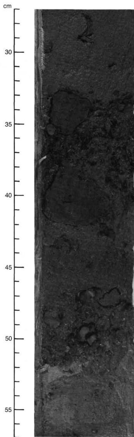
Figure 13. Erosional contact between silty muds (top and bottom). The transition zone consists of dark olive gray to black phosphatic sand and phosphatic nodules. The top of the underlying section shows burrows filled with phosphatic sand (Sample 112-687B-3H-5, 27–57 cm).
