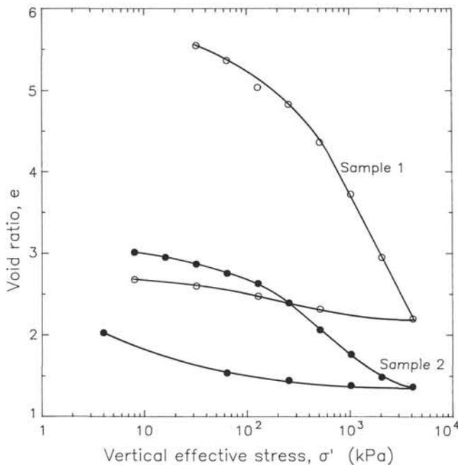
Figure 2. Void ratio vs. log effective vertical stress for Samples 1 and 2. Sample 1 exhibits the higher initial void ratio and higher compression index, reflecting the differences in the two samples.
