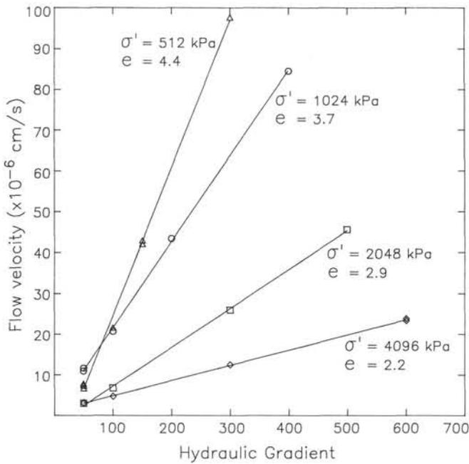
Figure 3. Flow velocity vs. hydraulic gradient for Sample 1. The four curves are for four different void ratios.
