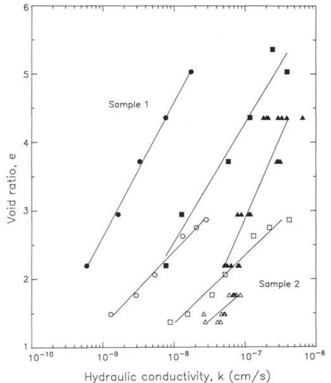
Figure 5. Void ratio vs. hydraulic conductivity for Samples 1 and 2. Sample 1 data are shown as solid symbols, while Sample 2 data are shown as open symbols. Three types of data are shown for each sample. The  $k$  was calculated from the log time (shown as circles) and root time (shown as squares) consolidation data as well as measured directly from the constant-head test (shown as triangles).
