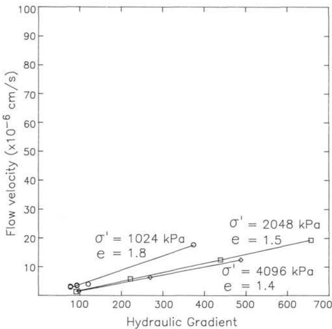
Figure 4. Flow velocity vs. hydraulic gradient for Sample 2. The three curves are for three different void ratios.
