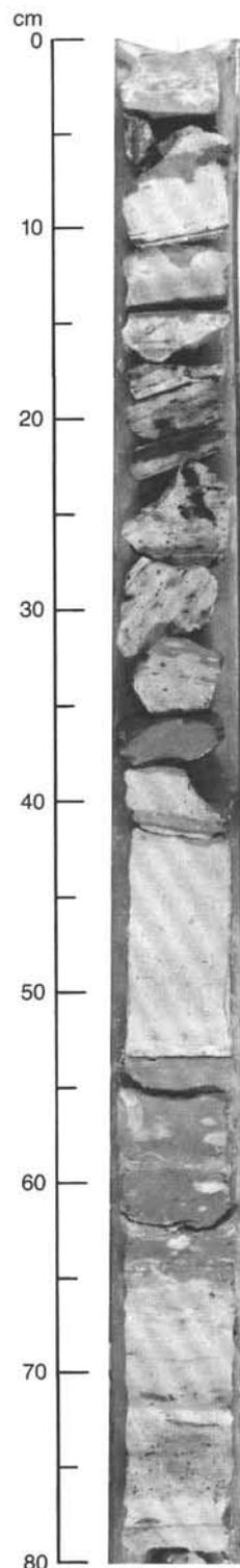
Figure 8. An example of the mixed, interbedded lithologies characteristic of Unit IV found in Section 115-707C-13R-1. From top to bottom, these include chert (0–14 cm), foraminifer-bearing silicified limestone (14–23 cm), micritic chalk (23–38 cm), claystone (38–53 cm), micritic chalk (53–65 cm), and partially silicified limestone (65–80 cm).
