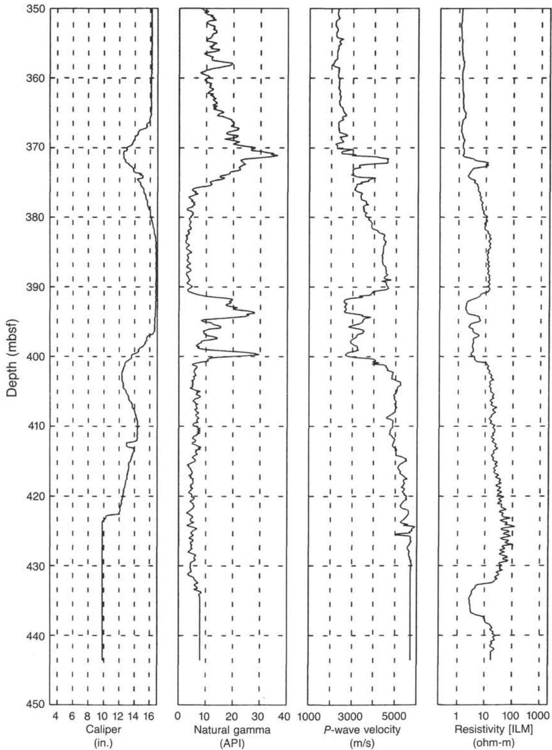
Figure 41. "Stacked" plot of caliper, natural gamma, *P*-wave velocity, and ILM resistivity for the interval from just above the sediment-basalt contact at 375 mbsf to the bottom of Hole 707C. Interbedded sediments are present from 392 to 401 mbsf and 433 to 437 mbsf.
