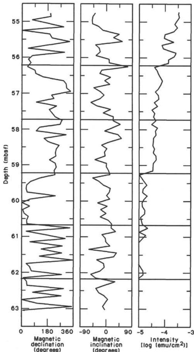
Figure 12. Pass-through magnetometer record from Core 115-707A-7H after demagnetization at 5 mT. Declination is given in core coordinates. Horizontal lines indicate section breaks.
