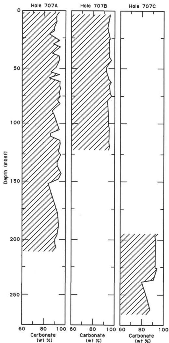
Figure 30. Carbonate content of samples for which the index properties were measured at Site 707.
