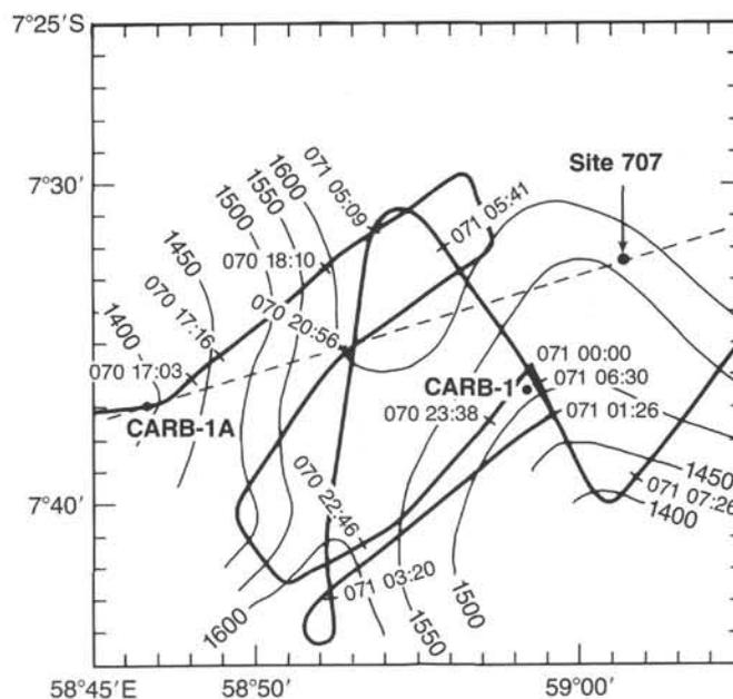
Figure 37. Bathymetry in the vicinity of Site 707 compiled from site survey data collected during the *Charles Darwin* cruise 21/87. The position of the *JOIDES Resolution's* approach and single-channel seismic (SCS) profile is also shown (dashed line). Depth in meters.
