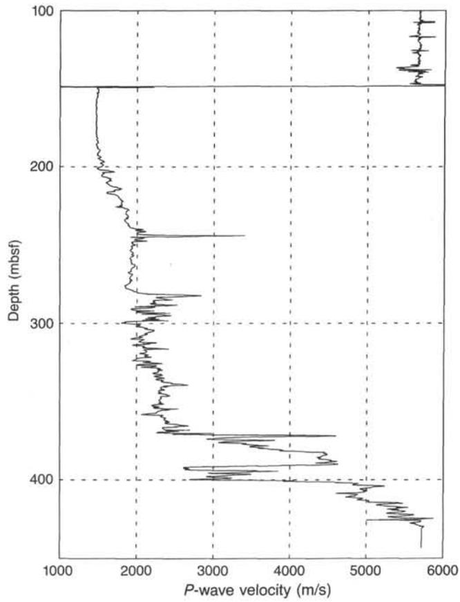
Figure 42. Compressional-wave velocity in m/s vs. depth below seafloor at Hole 707C.
