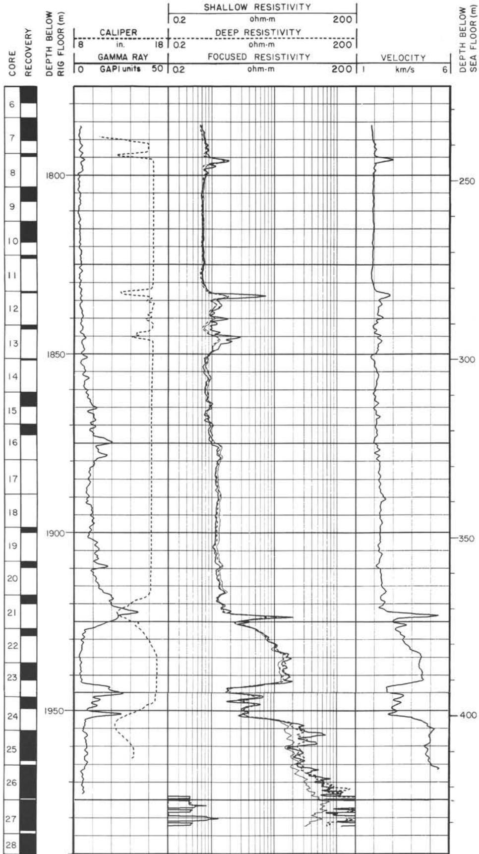
Figure 40. Summary log for Hole 707C. Caliper, natural gamma ray, resistivity (shallow, deep, focused), and traveltime (presented as seismic velocity) logs. Units and scales as shown on figure. Gamma-ray data in API (American Petroleum Institute) units.
