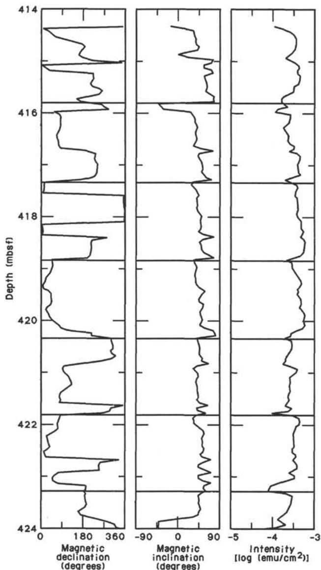
Figure 14. Pass-through magnetometer record from basalt Core 115-707C-26R after a demagnetization treatment of 9 mT. Conventions as in Figure 12.
