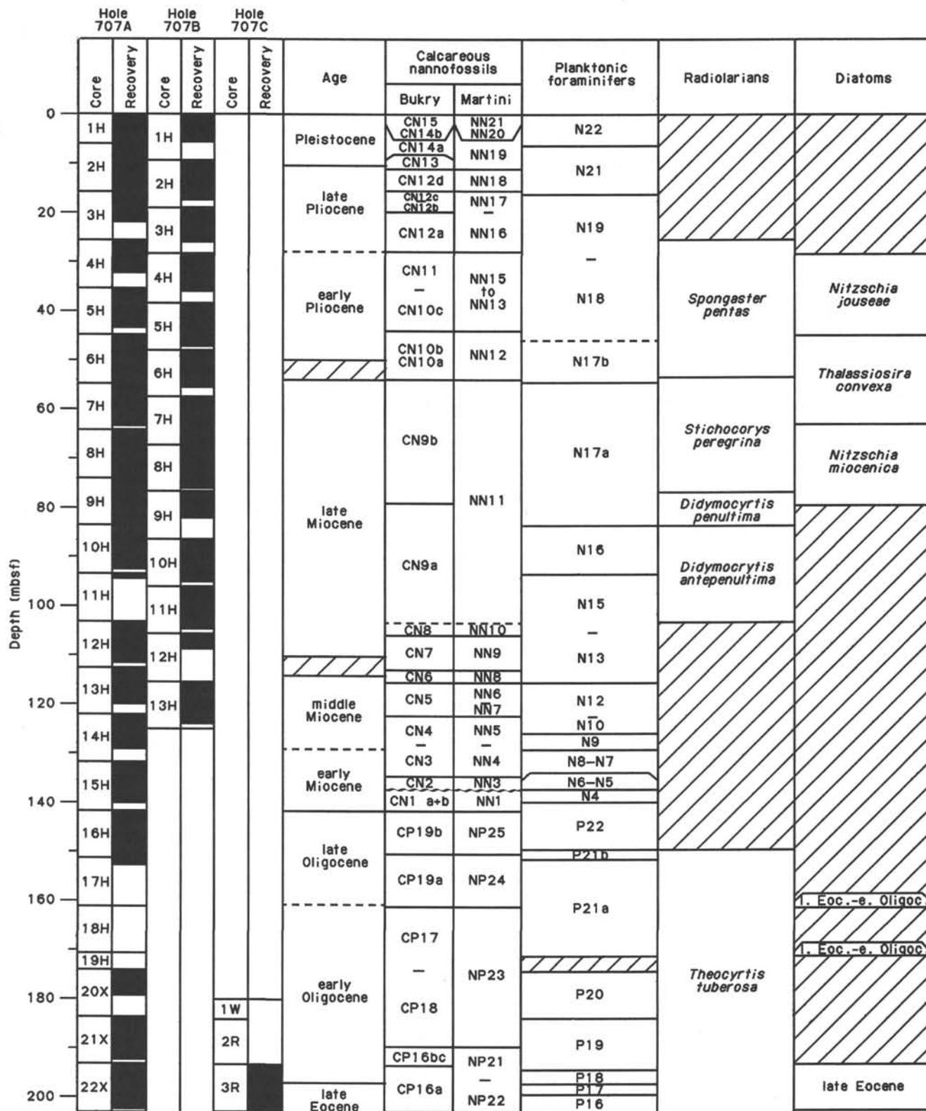
Figure 11. Biostratigraphic summary, Site 707, as based on Holes 707A (0–212.3 mbsf) and 707C (from 212.3 mbsf to basement).
