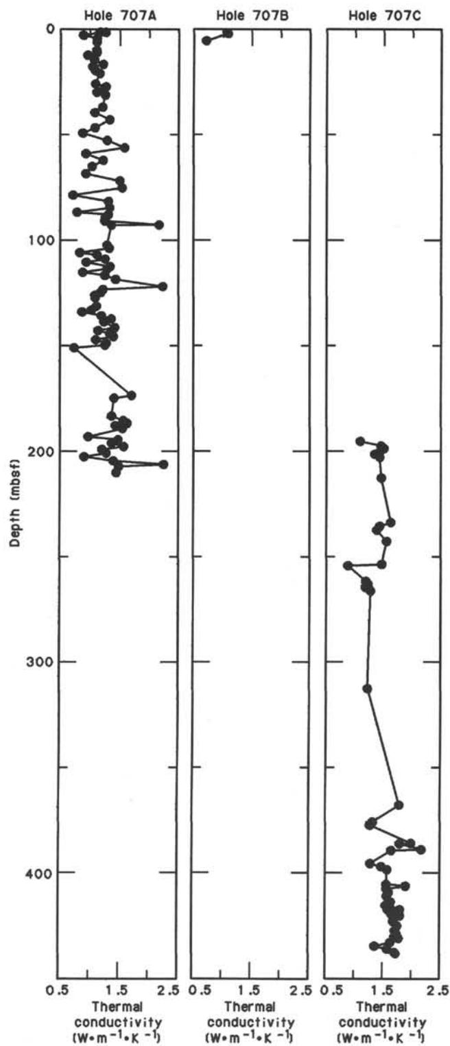
Figure 36. Thermal conductivity at Site 707.
