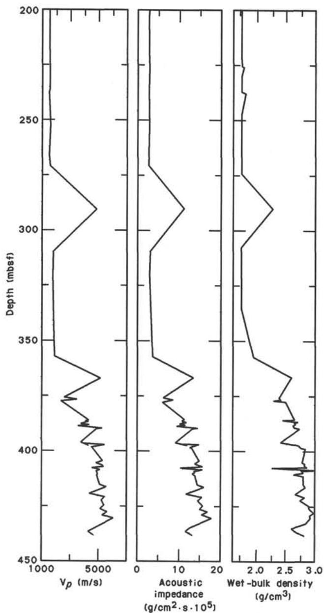
Figure 35. Compressional-wave velocity, acoustic impedance, and wet-bulk density in Hole 707C.
