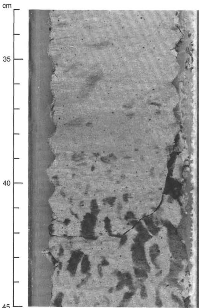
Figure 9. Evidence of bioturbation in a glauconitic foraminifer-bearing nannofossil limestone (Unit IV) from Section 115-707C-15R-3. Preserved burrow traces are enhanced by the presence of glauconite.
