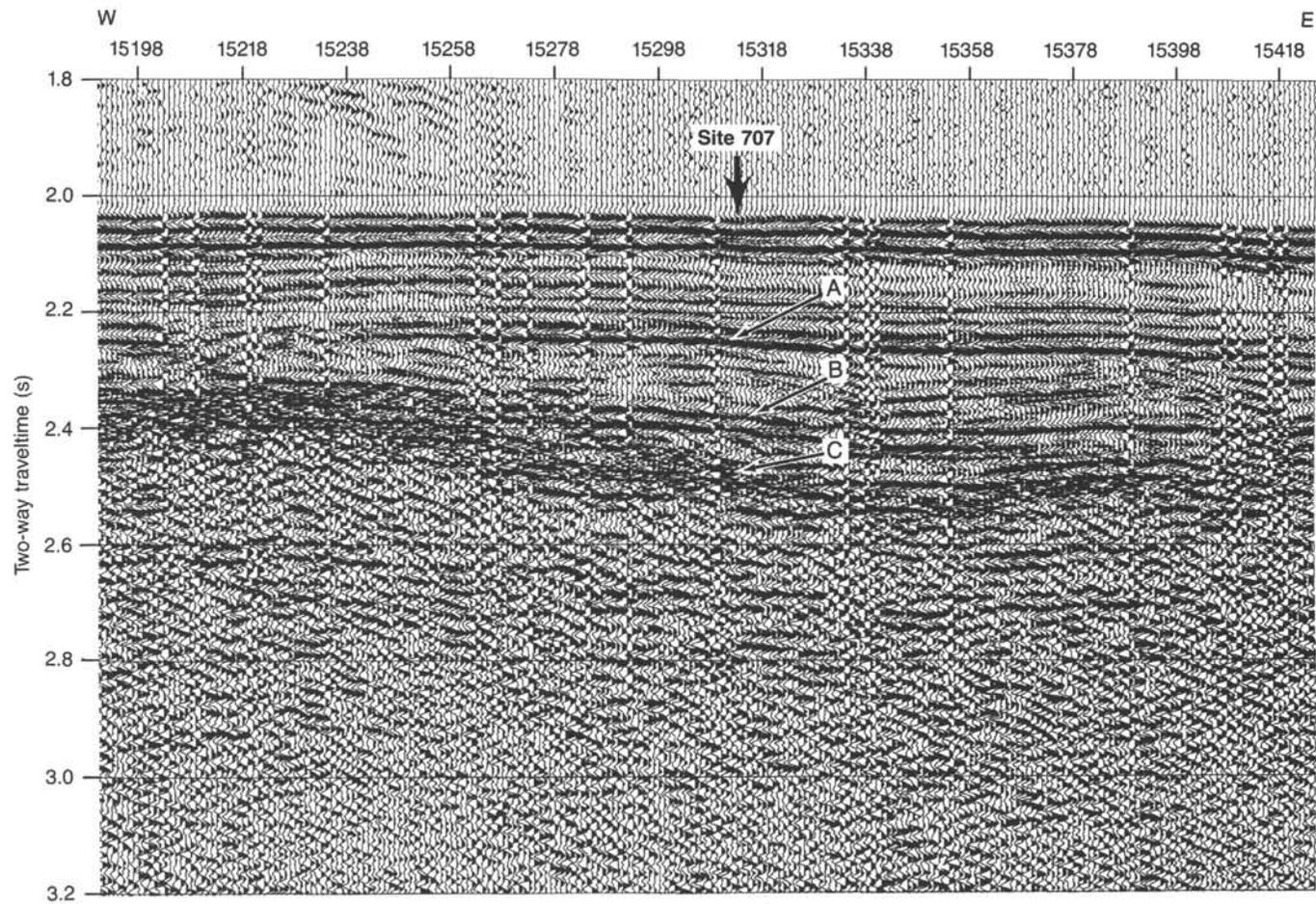
Figure 39. Seismic section at Site 707 produced from *JOIDES Resolution's* single-channel seismic (SCS) profile. A series of prominent reflectors are seen at 0.20 **A**, 0.32 **B**, and 0.41 **C** s (two-way traveltime) below the seafloor. The first two are related to impedance changes in the Cenozoic sedimentary section, the third is the basaltic basement.
