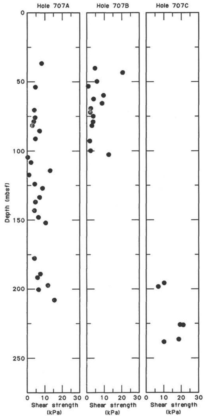
Figure 33. Shear strength at Site 707.
