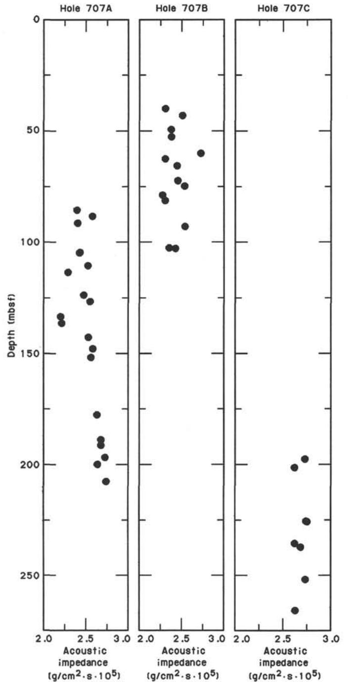
Figure 34. Calculated values of acoustic impedance at Site 707.
