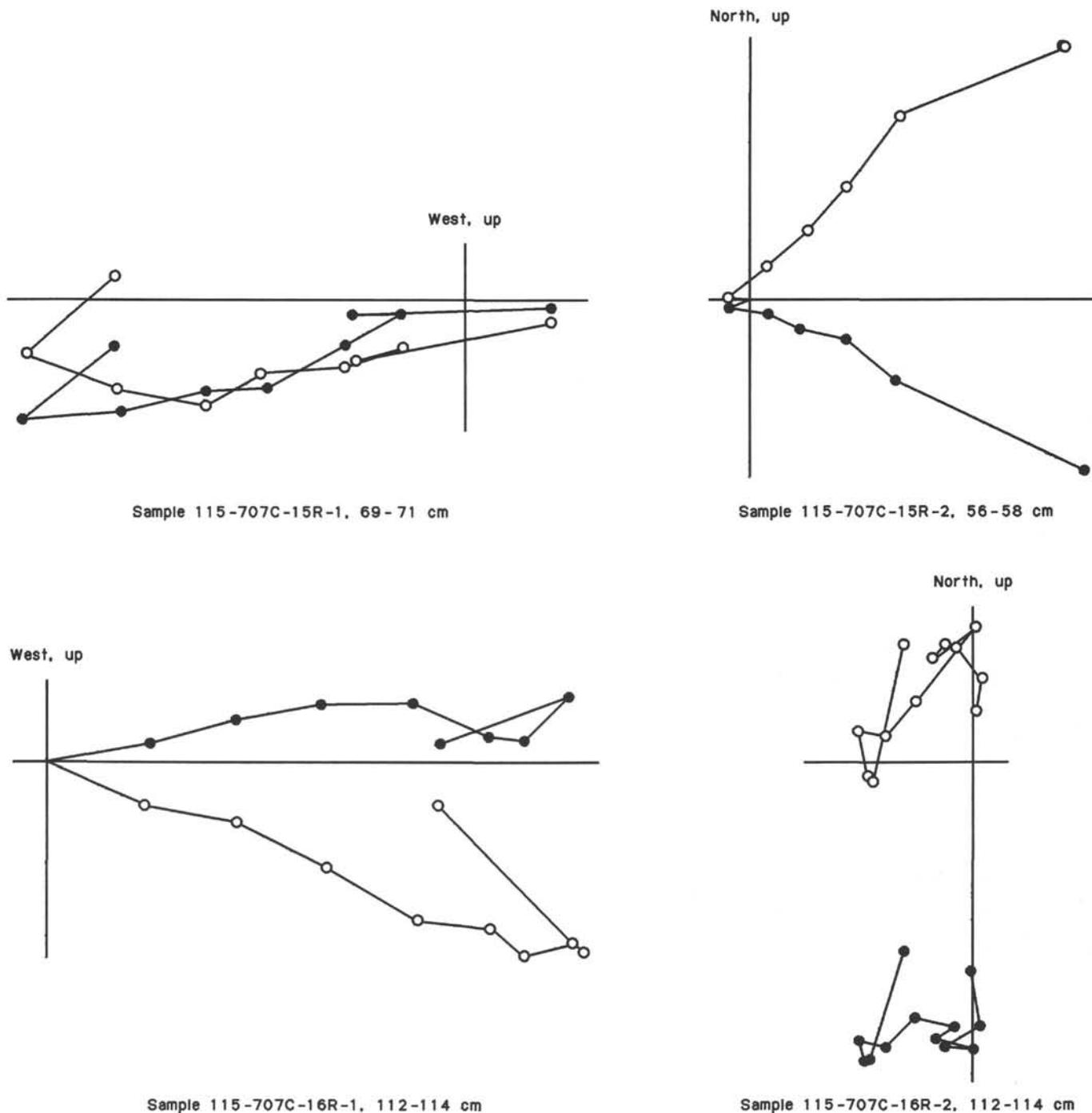
Figure 13. Zijderveld orthogonal projection diagrams of glauconitic sediment samples subjected to alternating-field (AF) demagnetization. Open points represent projection in the vertical plane; closed points, in the horizontal plane.
