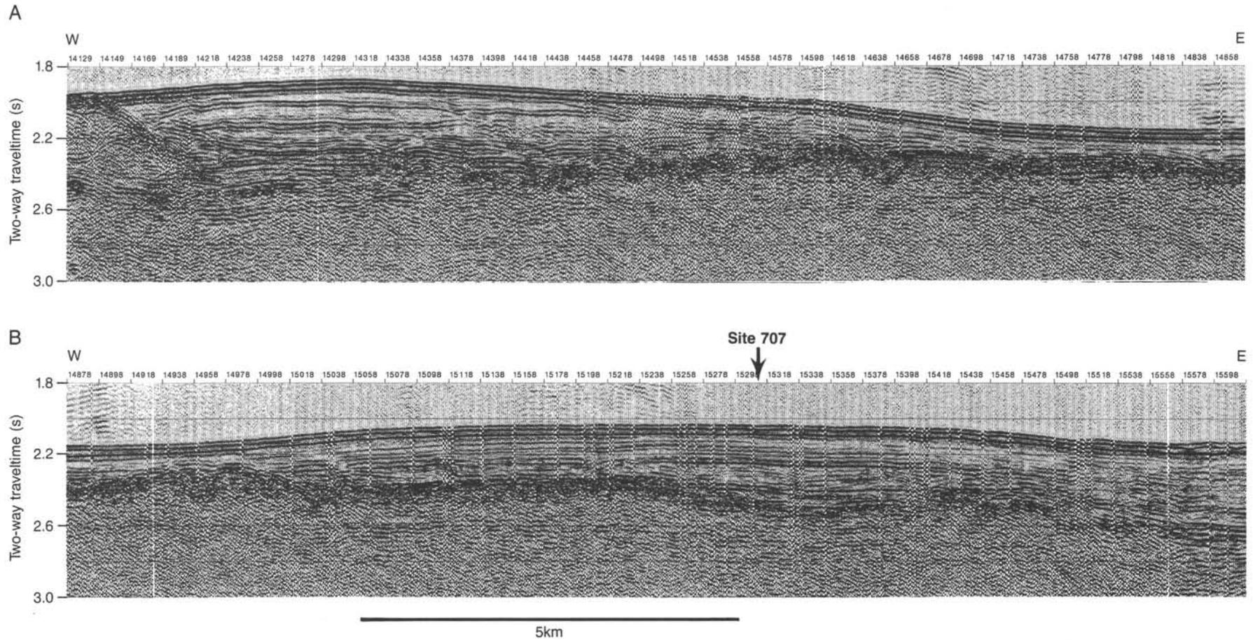
Figure 38. Single-channel seismic (SCS) survey conducted by the *JOIDES Resolution* through Site 707. The profile (located in Fig. 37) is along a west to east section across the top of the ridge which connects the Seychelles Bank and the Saya de Malha Bank (**B** follows to the east of **A**). Site 707 is located over a small sedimentary basin formed by slight offsets (probably normal faults?) in the basement.
