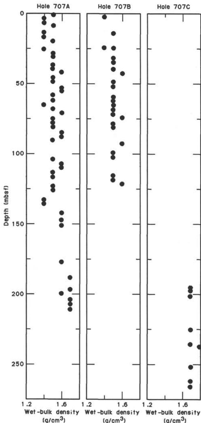
Figure 27. Wet-bulk density at Site 707.
