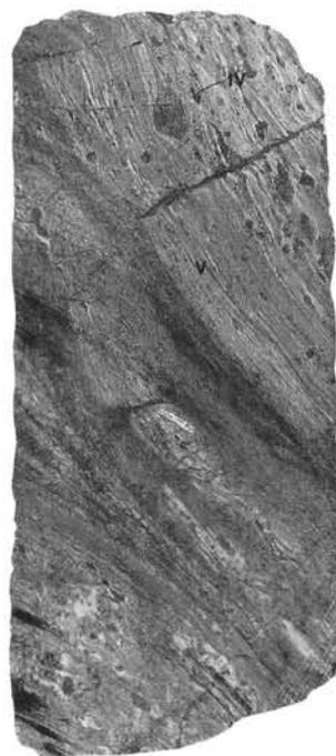
Figure 6. A decimeter-thick mylonitic shear in textural Type IV gabbros. Sample 118-735B-2D-1, 134–149 cm. Ruler is vertical and points upward. Stretching lineation is down-dip. Roman numerals represent textural types (see text).
