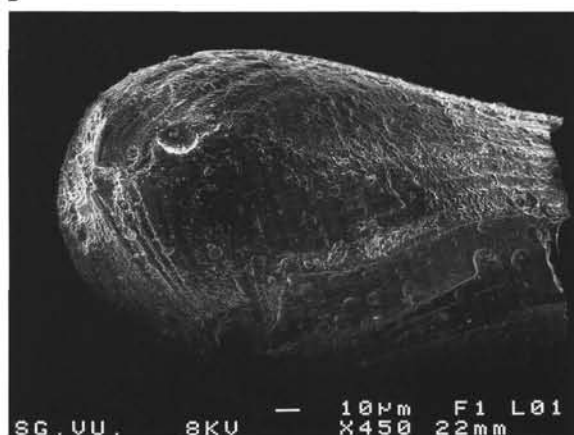
Figure 4. SEM photomicrographs of microtektite droplets from Sample 121-758B-1H-1, 141–143 cm. All three show flowlines on the surface of the microtektites.
