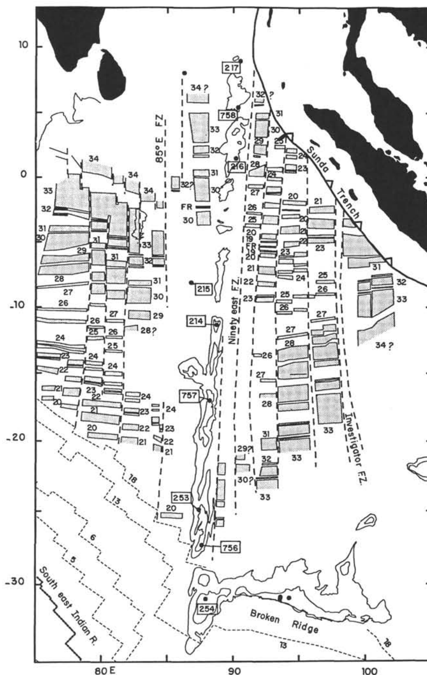
Figure 2. Tectonic chart of the Central Indian Basin and Wharton Basin. Shaded rectangles correspond to normal reversals recorded by the ocean floor; numbers refer to the magnetic chrons. Fossil ridges (extinct spreading-ridge segments) are labeled FR and represented by heavy lines. Heavy dashed lines outline the fracture zones (F.Z.'s); light dashed lines are isochrons (Chrons 5, 6, 13, and 18; after Royer and Sandwell, 1989).
