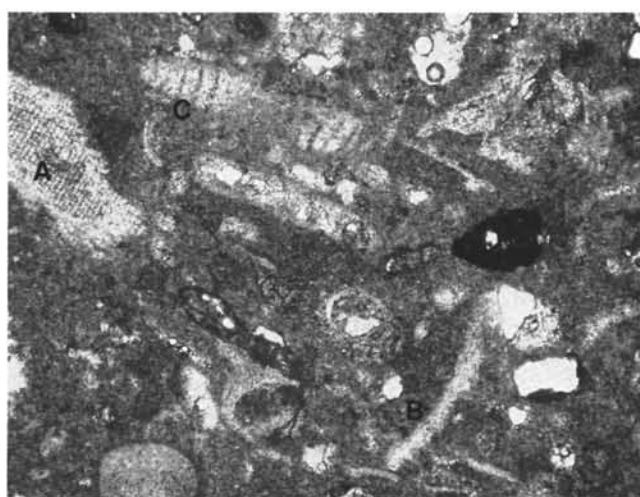
Plate 4. Thin-section photomicrographs of Unit VI lithology, Site 764. 1. Sample 122-764B-21R-CC, 26–28 cm. Dolomitized packstone to grainstone. Zoned dolomite (A) surrounding pelmatozoan fragment (B). Note dolomite replacing pelmatozoan fragment. Dark areas between dolomite grains are filled with limonite. 2. Sample 122-764B-25R-1, 14–16 cm. Boundstone to rudstone. Large coral fragment (A) and coralline algae(?) allochem (B) with micrite between allochems. Bright areas on slide are pore spaces producing a vuggy texture. 3. Sample 122-764B-26R-1, 13–16 cm. Grainstone. Large mollusk fragment (A) surrounded by micritic envelope and internal neomorphic sparite. Pelmatozoans (B) with syntaxial overgrowths being dissolved and replaced with pore-filling calcite (C). Algal fragments in areas (D) and (E). Note overly close packing and embayed grains. 4. Sample 122-764B-26R-1, 19–21 cm. Wackestone to packstone within large coral boundstone. Allochemical grains include pelmatozoans (A), mollusk (B), and algae (C). Micrite matrix shows patchy recrystallization and moldic (vuggy) texture.
