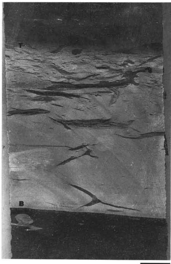
Figure 4. Base-cut-out fine-grained turbidite ( T_2 in Fig. 3) lacking lower parallel laminated division. Turbidite consists of clay, nannofossils, micrite, and lesser calcispheres and radiolarians; note sharp base (B), gradational top (T), and downward decrease in bioturbation. 123-765C-57R-2, 80–89 cm; scale bar is 1 cm.
