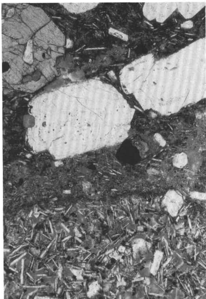
Figure 45. Intersertal textured andesite xenolith within porphyritic andesite. Sample 126-792E-71R-3, 33–34 cm, Unit 1. Plane polarized light, 95 \times .
