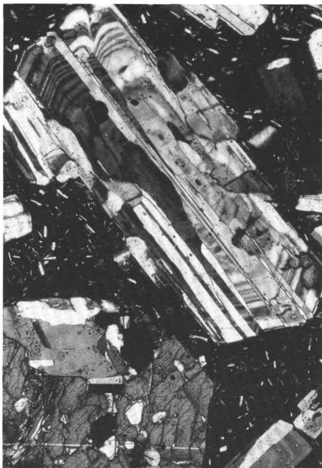
Figure 43. Typical texture of the porphyritic andesite. Oscillatory zoned plagioclase and euhedral clinopyroxene in a microphyric groundmass of feldspar and glass. Section 126-792E-71R-CC, Unit 1. Cross-polarized light, 95 \times .
