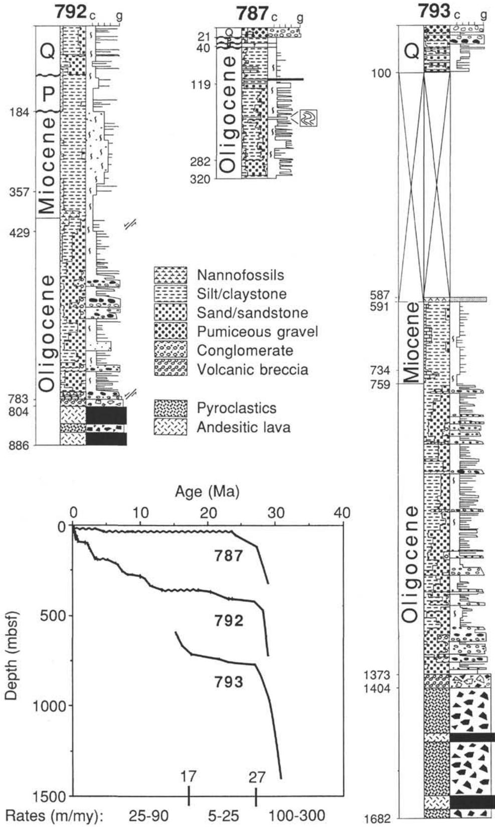
Figure 7. Lithostratigraphic summaries for Leg 126 forearc Sites 787, 792, and 793. The depths (mbsf) of unit boundaries are shown on the left of each column and a graphic sedimentological log displays the relative grain size on the right (from c = clay to g = gravel). An age-depth plot, showing three periods of distinct sedimentation rates, is shown on the bottom left.
