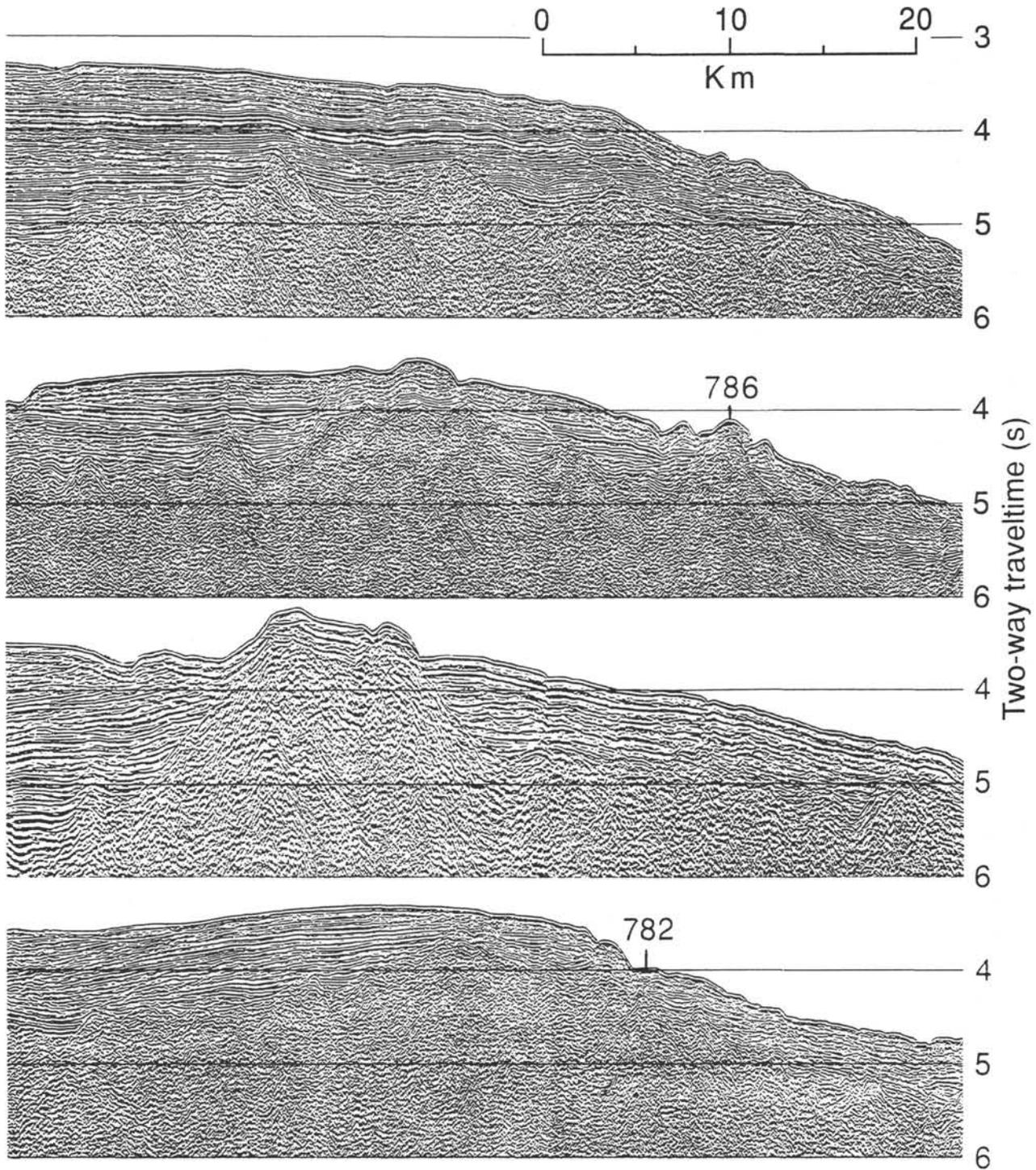
Figure 4. Hawaii Institute of Geophysics (HIG) migrated MCS profiles at 6.7 vertical exaggeration across the outer arc high near 32°N (top two profiles) and 31°N (bottom two profiles). See Figure 2 for location. Note the onlap of the forearc sediments onto the numerous basement protrusions, which I infer to be volcanic edifices similar to those drilled at Sites 782 and 786.
