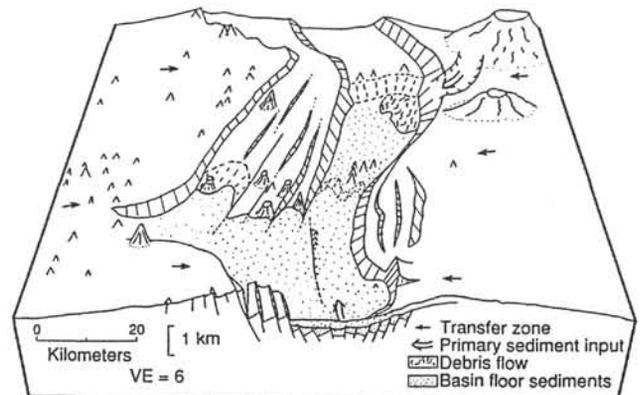
Figure 17. Perspective block diagram of the Sumisu Rift, viewed from an elevation of 65°, looking 345°, and with a vertical exaggeration (VE) of 6 (after Klaus et al., this volume, and B. Taylor et al., 1991).
