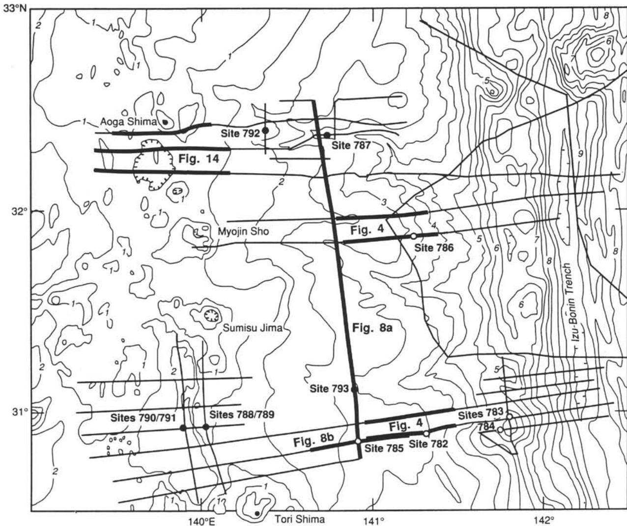
Figure 2. Locations of U.S. multichannel seismic profiles and Sites 782-786 (Leg 125) and 787-793 (Leg 126) in the Izu-Bonin region. The bathymetric base map is contoured at 500-m intervals and labeled in kilometers. Bold MCS profile segments are shown in Figures 4, 8, and 14.
