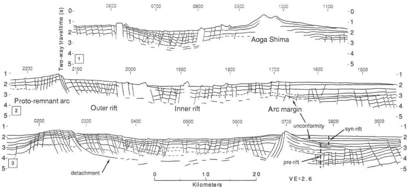
Figure 14. Line drawings of migrated MCS profiles across Aoga Shima Rift (see Fig. 2 for locations) after Klaus (1991). VE = vertical exaggeration.
