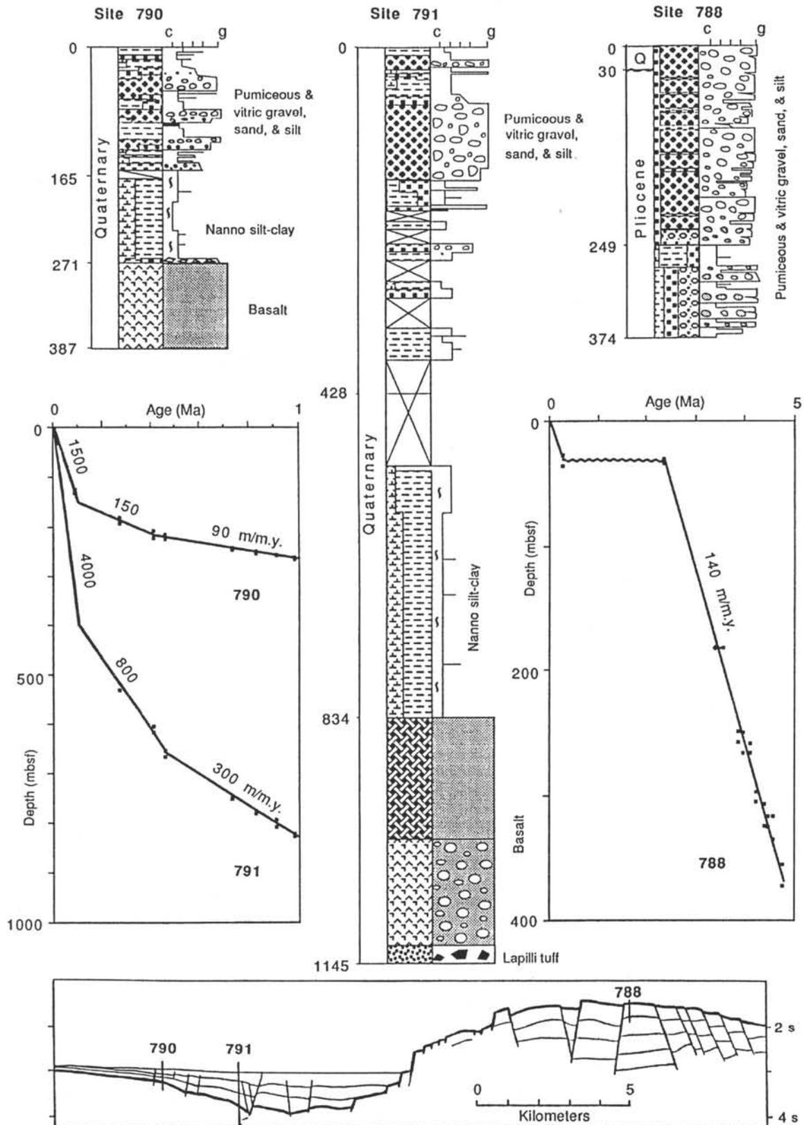
Figure 18. Lithostratigraphic summaries for Leg 126 Sumisu Rift Sites 788, 790, and 791. The depths (mbsf) of unit boundaries are shown on the left of each column, and a graphic sedimentological log displays the relative grain size on the right (from c = clay to g = gravel). Age-depth plots are shown in the center, with uncorrected sedimentation rates labeled in m/m.y. A simplified line drawing of MCS Profile 4 (Fig. 16) is shown with site locations at the bottom.
