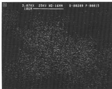
Plate 5. Authigenic harmotome in ash layer 9-209 (Section 128-799B-27R-5 at 47-51 cm). 1. Harmotome crystals growing in glass. 2, 3. Glass shard, X-ray distribution pattern of Ba.
