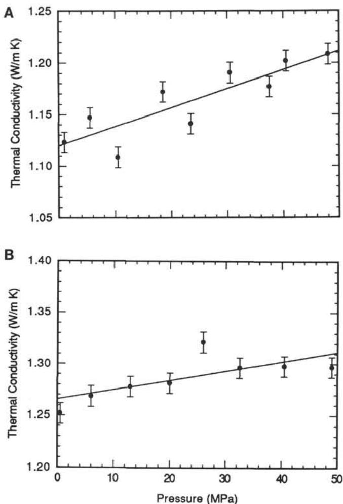
Figure 1. Mean thermal conductivity of core samples vs. hydrostatic confining pressure with the estimated probable error of 0.01 W/m · K. Solid line is the least-squares fit to a straight line. A. Sample 131-808A-9H-2, 113–120 cm. B. Sample 131-808B-7X-4, 49–55 cm.
