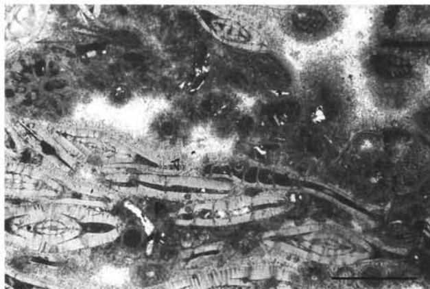
Figure 8. Bryozoan–larger foraminifer microfacies (MF3). Well-cemented grainstone showing early marine fibrous cement and a second generation of scalenohedral calcite. Scale bar = 0.5 mm (Sample 133-825B-7R-1, 68–71 cm).
