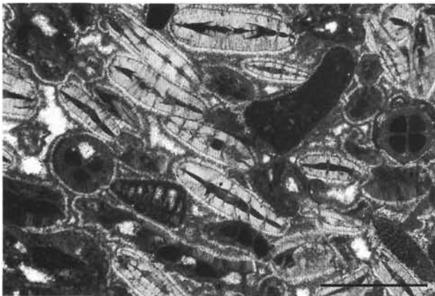
Figure 6. Bryozoan–larger foraminifer microfacies (MF3). Bioclastic grainstone consisting mainly of larger foraminifers ( Operculina ) and branching bryozoans (ERro) with few partly rounded limestone lithoclasts. Chambers of foraminifers and zoecias of bryozoans are filled with microbioclastic micrite. Interparticle voids are lined by two generations of equant marine cement and scalenohedral calcite cement. Scale bar = 0.5 mm (Sample 133-824C-8R-1, 61–63 cm).
