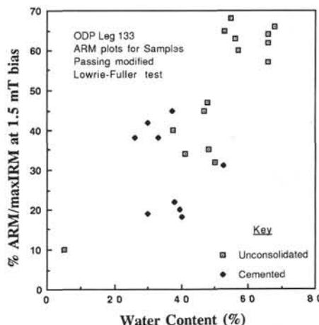
Figure 10. Plot of ARM acquisition value at 1.5 mT vs. natural water content determined from shipboard analysis. The degree of magnetostatic interaction appears to be correlative with porosity reduction through formation of cement crystals.
