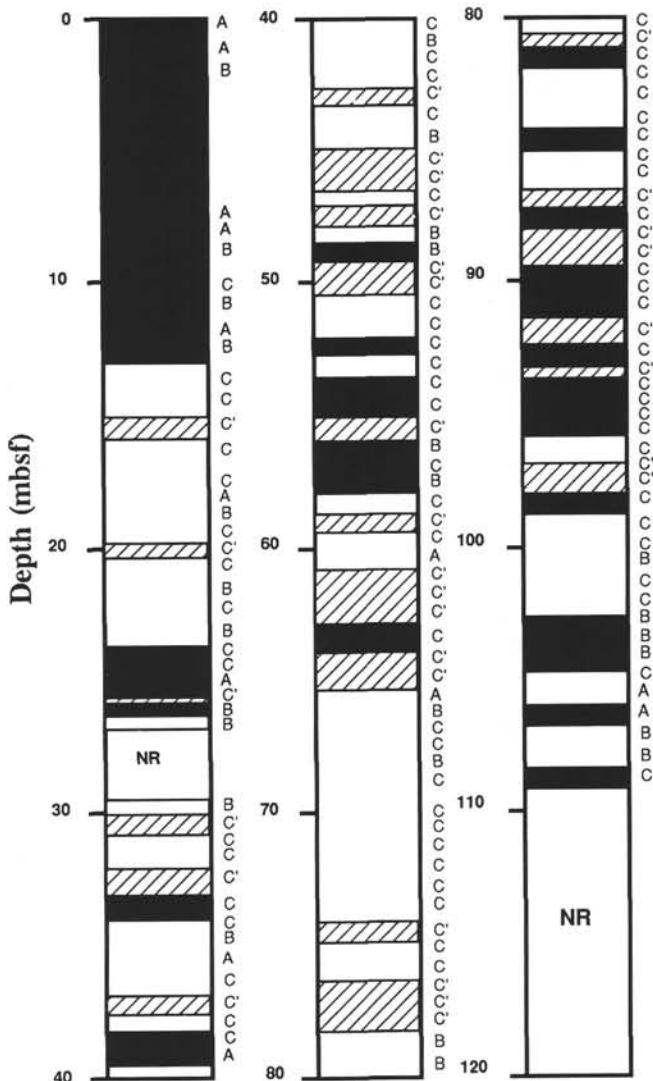
Figure 15. Summary of magnetic polarity zones and distribution of paleomagnetic samples for Holes 812A and 812C. The low magnetic intensity and instability of many C and C' samples precluded assignment of polarity zones below the upper 30 mbsf.
