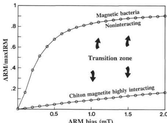
Figure 9. End-member calibration of noninteracting, single-domain magnetite from freeze-dried bacteria and highly interacting magnetite from chiton teeth. Recent work involves calibration of the intermediate transition zone between the two (McNeill et al., 1991).
