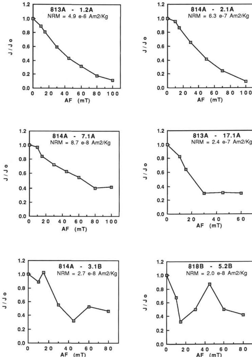
Figure 6. Typical  $J/J_0$  plots from carbonate samples at Sites 812 through 814. Most samples responded to AF demagnetization. Magnetically weak and unstable samples often showed irregular patterns with increasing AF demagnetization.
