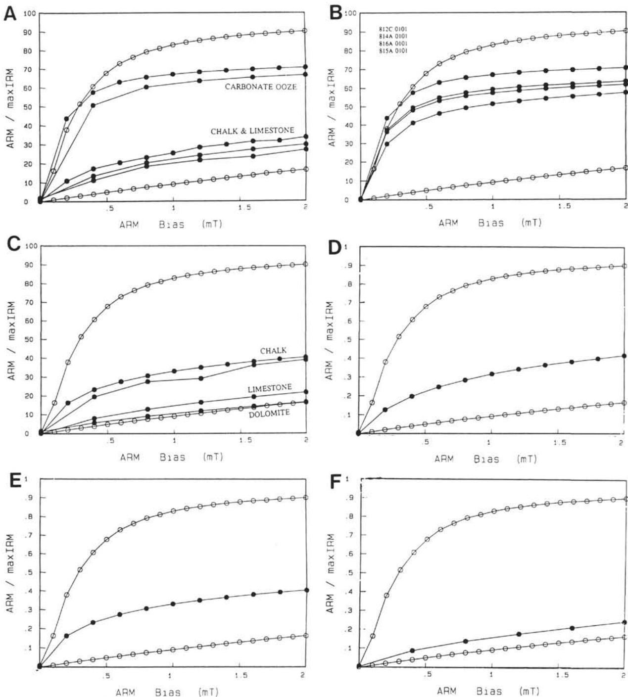
Figure 8. ARM plots of carbonate samples from the Queensland Plateau. Near-surface samples exhibit a highly noninteracting configuration, which suggests a biogenic magnetite source. **A.** Hole 814A, 3H-2. **B.** As shown. **C.** Site 817. **D.** Hole 818B, 6H-1. **E.** Hole 817C, 5H-1. **F.** Hole 812C, 12H-CC.
