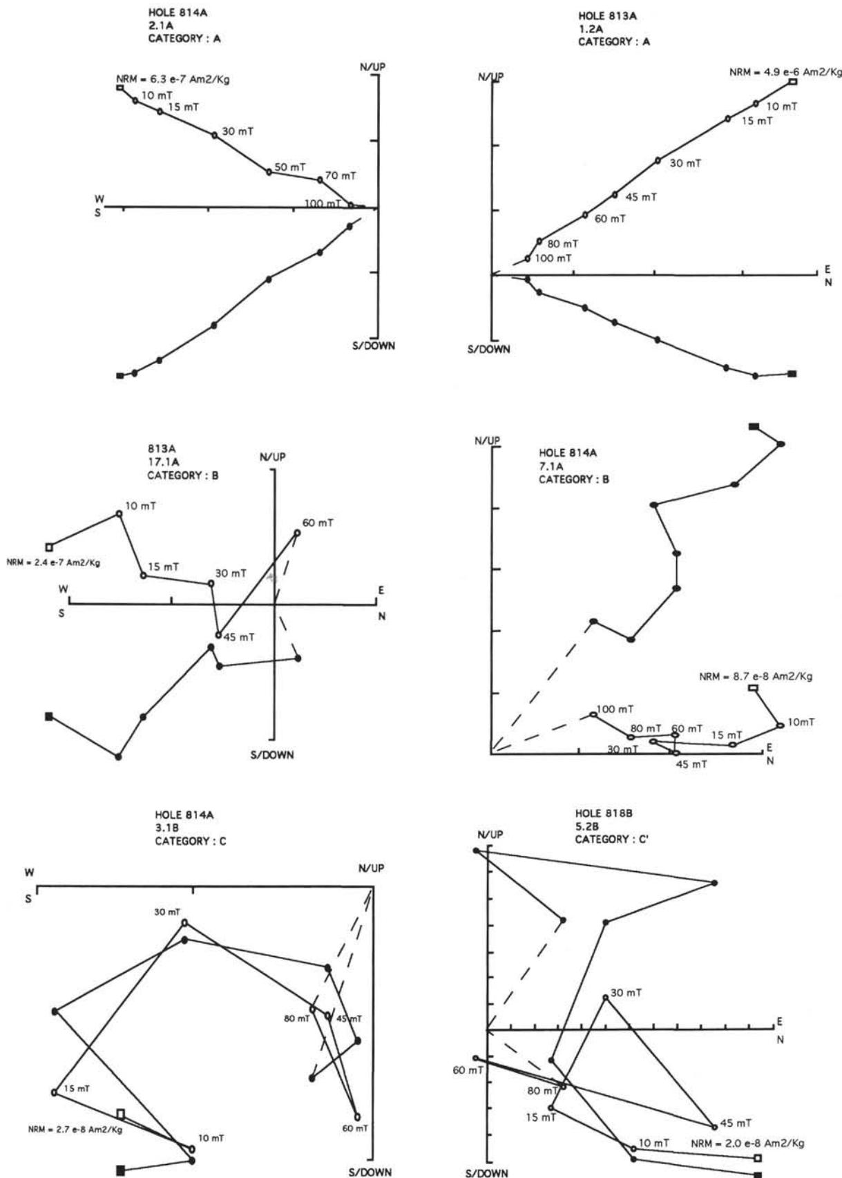
Figure 14. Representative orthogonal plots of A, B, C, and C' samples from the carbonate sediments of the Queensland Plateau. Most samples fell under the C or C' category and generally were unusable for magnetostratigraphic purposes.
