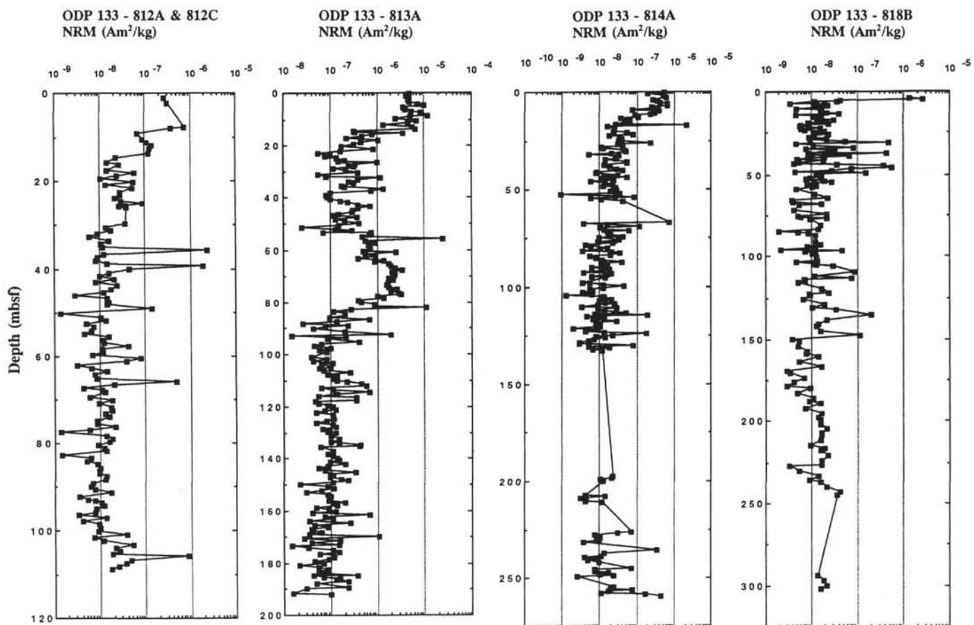
Figure 3. Summary of NRM intensities from Sites 812 through 814 and 818, measured from discrete samples in a magnetically shielded environment. NRM moments usually show a transition from higher intensity near the top of the core, to significantly lower intensity downcore.
