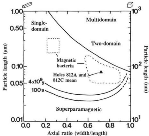
Figure 12. Mean crystal dimensions for 26 grains plotted on the stability diagram of Butler and Banerjee (1975). The size range is similar to that of known biogenic magnetite compiled by McNeill et al. (1988).
