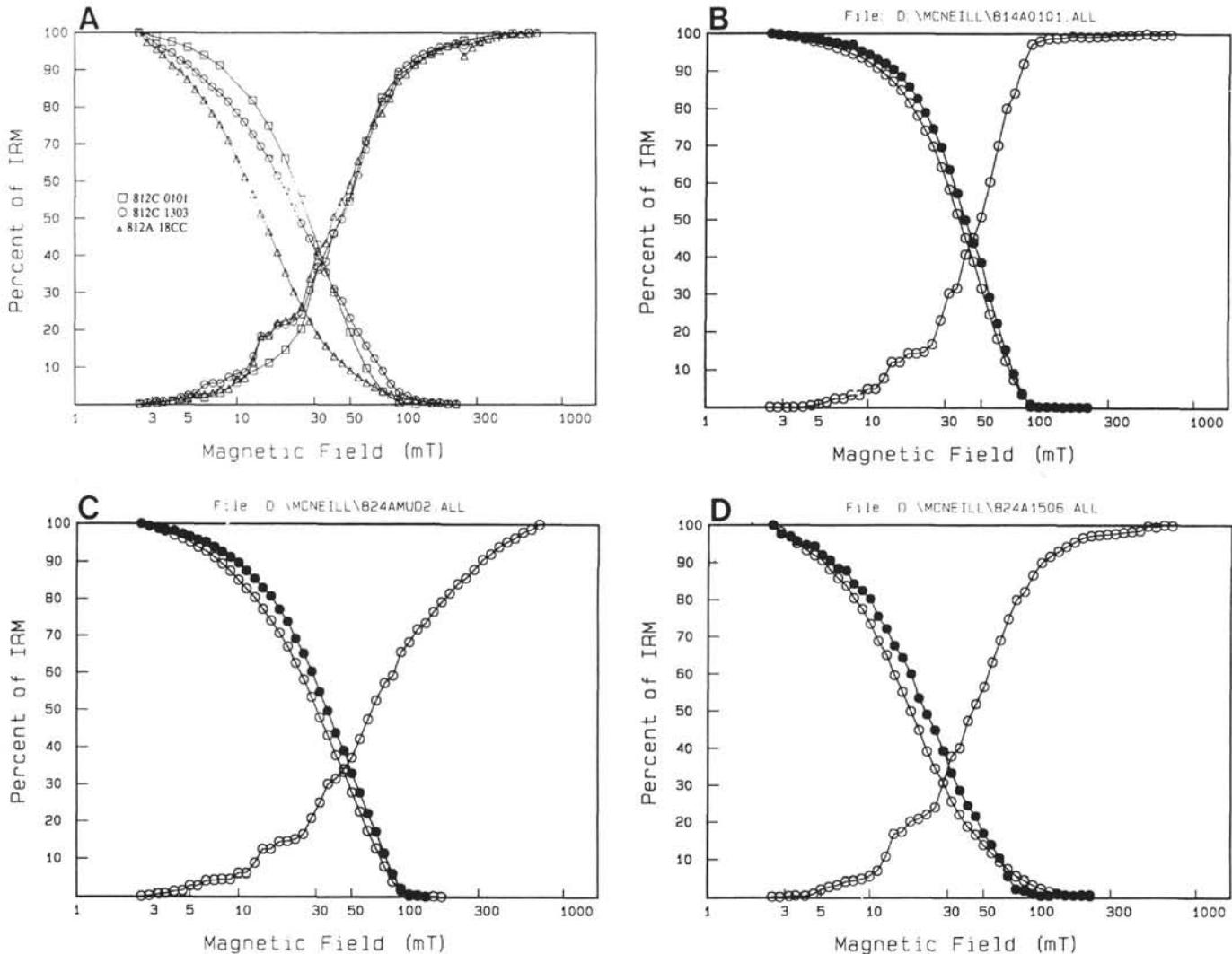
Figure 7. Coercivity spectral analysis plots of carbonate samples from the Queensland Plateau. Samples from Plateau Sites 812 through 814 passed the modified Lowrie-Fuller test, which suggests a single-domain magnetite/maghemite remanence carrier. **A.** Site 812. **B.** Hole 814A, 1H-1. **C.** Hole 824A mudline. **D.** Hole 824A, 15H-6.
