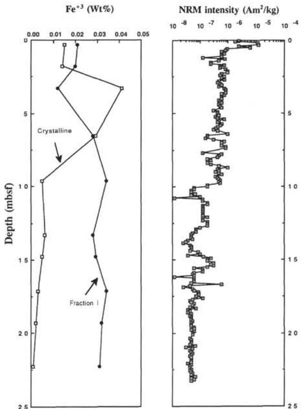
Figure 13. Summary of iron geochemistry and magnetic intensity from Hole 812A. Post-depositional alteration may have had significant effect on grain preservation and the ability to carry a stable magnetic remanence.
