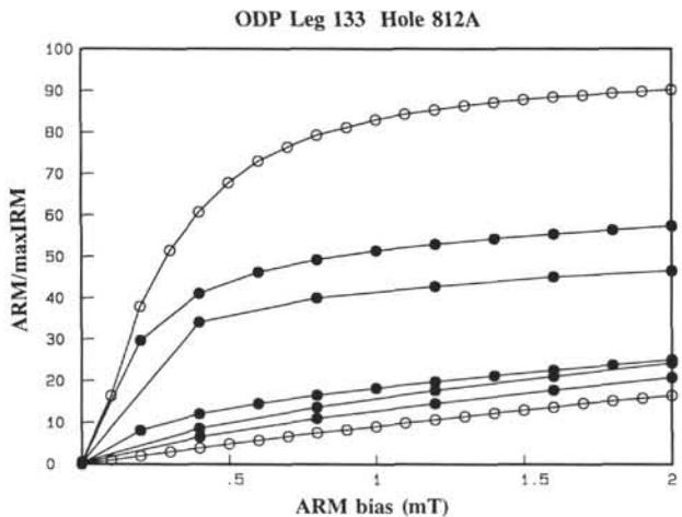
Figure 20. ARM acquisition plot showing the transition from more noninteracting unconsolidated sediments to a more interacting magnetostatic configuration with progressive cementation.
