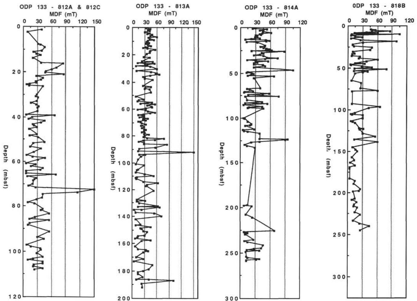
Figure 16. Downcore plot of median destructive field (MDF) after AF demagnetization. Most samples responded to progressively increased AF field demagnetization.
