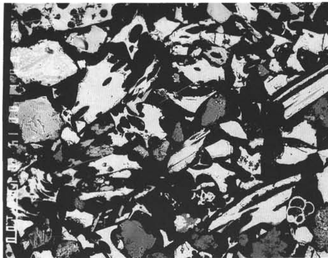
Figure 8. Back-scattered electron photomicrograph of volcaniclastic rock from Unit III. Note poor sorting and immature composition with angular and broken glass shards, igneous minerals, and rock fragments and biogenic grains. Scale bar = 100 \mu m. Sample 135-840B-60X-1, 72–77 cm.
