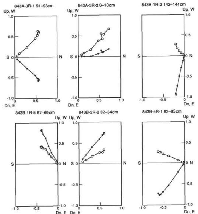
Figure 10. Normalized orthogonal demagnetization diagrams showing results of progressive stepwise alternating field demagnetization of basalt samples from Holes 843A and 843B. Demagnetization steps shown are NRM (0), 2.5, 5, 7.5, 10, 20, and 25 mT. Open circles are in the vertical plane, and filled circles are in the horizontal plane.
