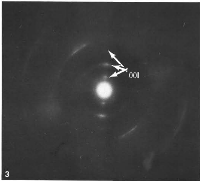
Plate 1. The selected area electron diffractions of minerals. 1. Todorokite with weak degree of structural perfection. 2. Asbolane-buserite. 3. Buserite-II. 4. Iron-vernadite.
