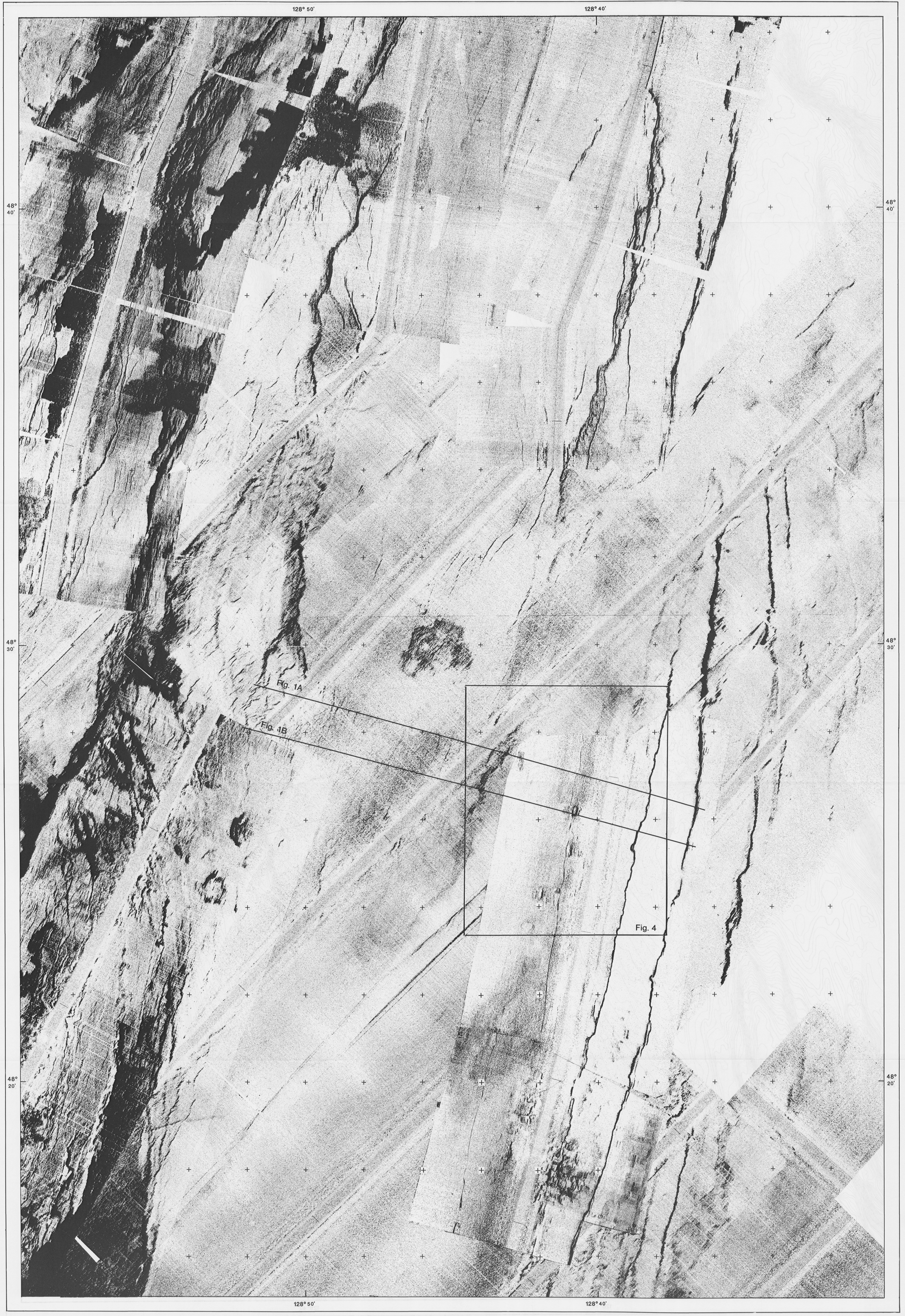
Figure 3. C. SeamARC II (12 kHz) acoustic image mosaic of the southern part of Middle Valley (from Davis et al., 1987). Areas of rough seafloor that cause high-intensity backscatter and steep slopes facing the side-scanning towfish are shown dark; acoustic shadows and areas of smooth seafloor are shown light. The area included in Figure 4 and the locations of the seismic reflection profiles shown in Figure 1 are indicated.
