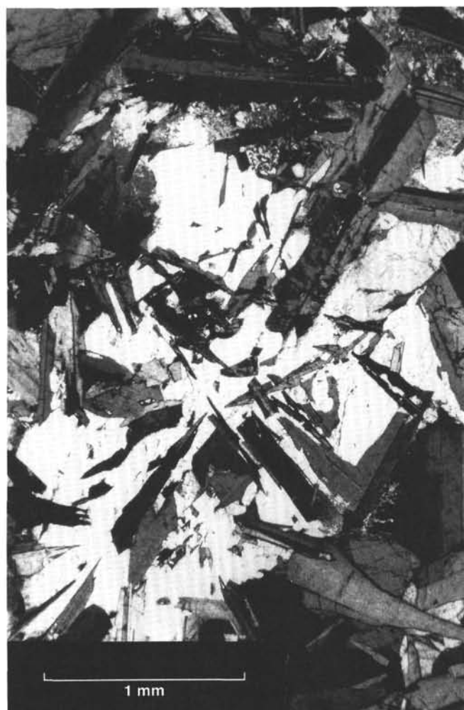
Figure 18. Anhedral, poikilitic augite with groundmass plagioclase chadacrysts in Sample 140-504B-199R-1, 105–110 cm.
