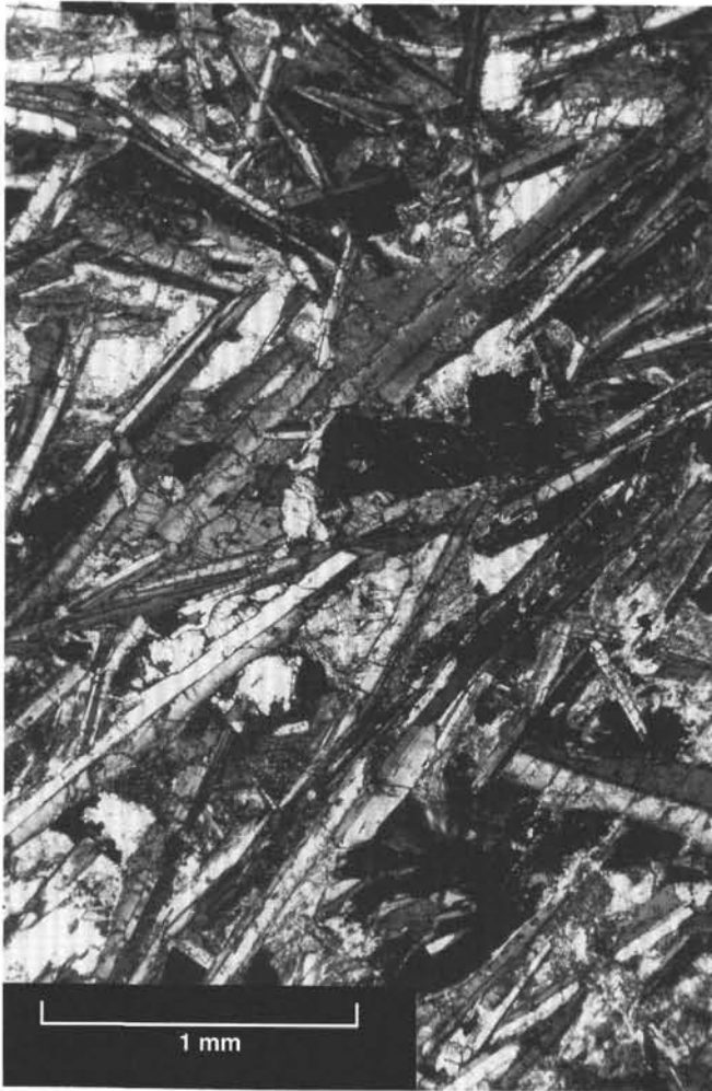
Figure 69. Preferred orientation of plagioclase groundmass laths in Sample 140-504B-186R-1, 53–57 cm (Piece 10). Cross-polarized light.
