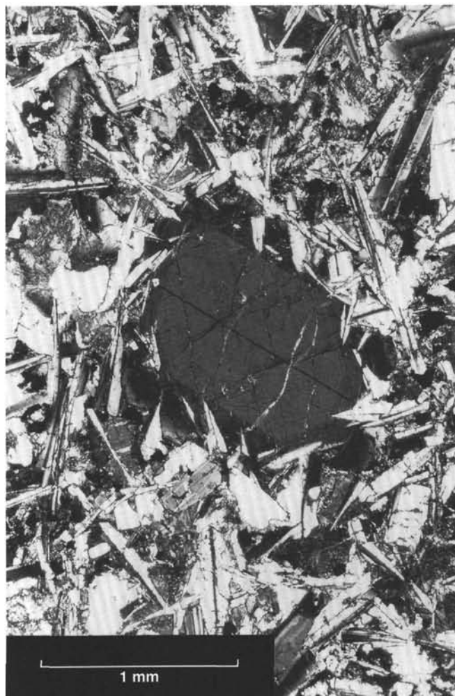
Figure 14. Normally zoned Cr-augite phenocryst showing ophitic overgrowth in Sample 140-504B-181M-2, 40–44 cm.
