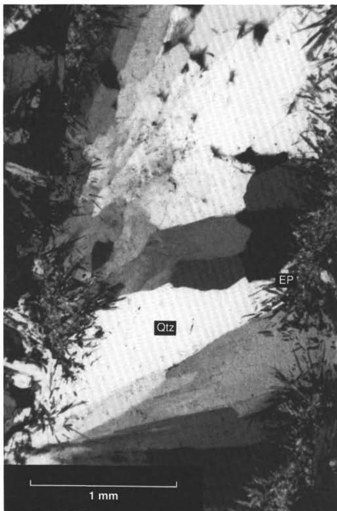
Figure 79. Quartz crystals arranged obliquely to the vein edges in a quartz-epidote vein (Sample 140-504B-192R-1, 13–14 cm (Piece 4)). Photomicrograph: crossed polars. Qtz: quartz; EP: epidote.
