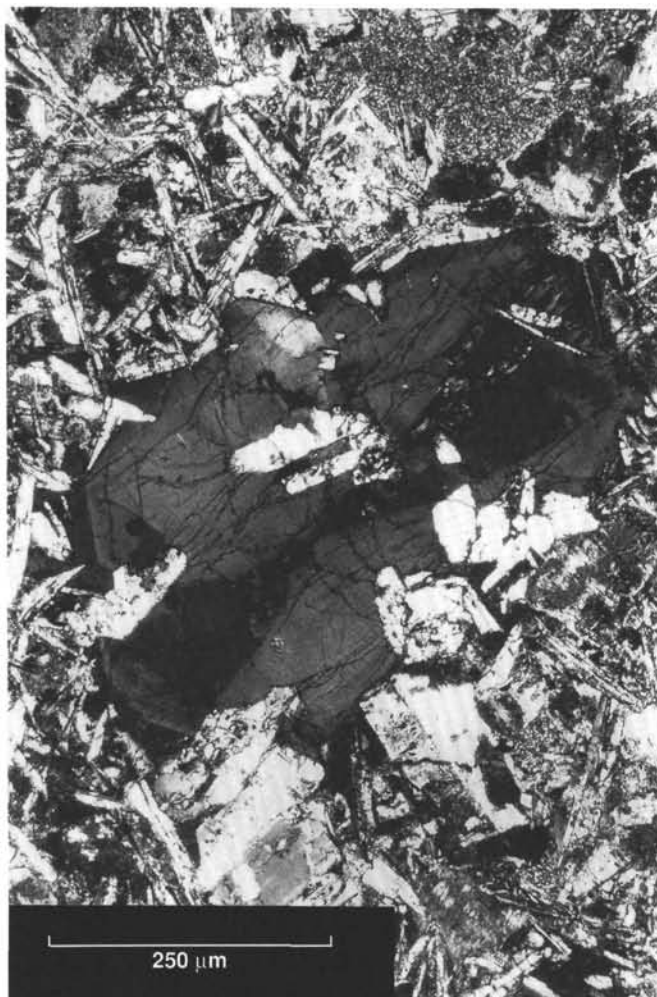
Figure 13. Sector-zoned Cr-augite phenocryst in Sample 140-504B-181M-2, 148–150 cm.
