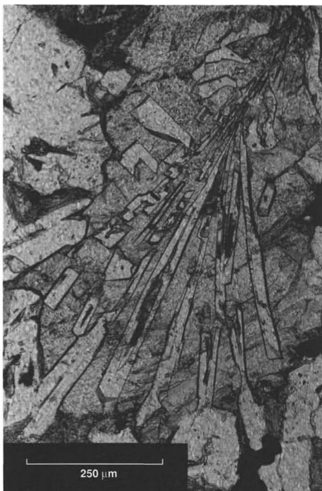
Figure 17. Branching groundmass plagioclase in Sample 140-504B-212R-1, 4–7 cm.
