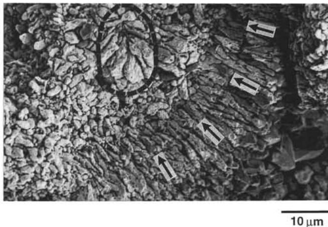
Figure 13. Spherulite (outlined) of probably microbial origin in micritic ooid core. Note well-developed epitaxial fringing cement with highly elongate crystals. Original ooid surface (arrow; SEM photograph, Sample 143-866A-139R-1, 21–22 cm; Subunit VIIC, Barremian).
