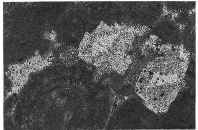
Figure 7. Grainstone with radial ooids and some void-filling and replacement dolomite. Dolomite rhombs have initially grown in pore space and then invaded ooids and peloids (Photomicrograph, plane light, Interval 143-866A-166R-1, 11–15 cm; scale 0.1 mm; Subunit VIIIA, Hauterivian).
