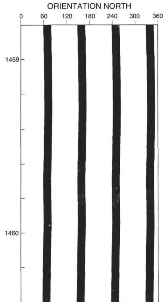
Figure 7. FMS image from 1458.8 to 1460.4 mbsf, Hole 866A. Dolomitization occurs preferentially within the most porous facies, the grainstones. In this example, some grainstone texture remains, although dark areas, corresponding to zones of higher porosity, cut across bedding planes.
