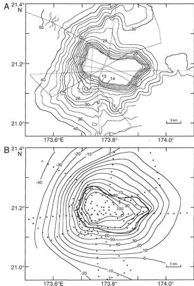
Figure 3. Bathymetry (A) and free-air gravity anomaly (B) maps of Heezen Guyot. Bathymetry contours are shown at 200-m intervals. Conventions are as in Figure 1.
