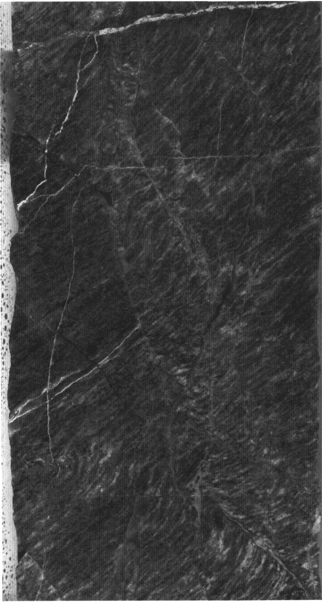
Figure 4. Typical foliation bands in the metamorphosed mafic rocks are discontinuous and fine, often being displaced and reoriented at fractures and veins, as observed in Sample 149-900A-82R-1, 100-111 cm. The foliation trend is variable and locally curved near fractures in a manner similar to drag folding.
