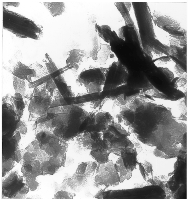
Plate 1. TEM pictures of clay fraction of samples from Atlantic City borehole, scale bar = 1 \mu\text{m} . 1. Sample 150X-AC-173-1394 (CMZ 6) showing abundant fleecy particles of I/S. 2. Sample 150XAC-93-755 (CMZ 4), authigenic smectite from sandy intervals. 3. Sample 150X-AC-36-193 (CMZ 2) euhehedral, hexagonal particles of kaolinite. 4. Sample 150X-AC-16-83 (CMZ 2) mixture of kaolinite and tubular particles of halloysite.
