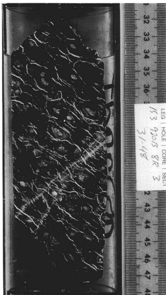
Figure 7. Discontinuous rings of fibrous chrysotile veins (V2) wrapping around the porphyroclasts in serpentized harzburgite. Some of these V2 veins are reactivated by massive wispy serpentine veins of the V3 generation that also crosscut at high angles a branching, aqua blue massive serpentine (V3) vein between 39 and 44 cm (Sample 153-920B-8R-3, 31–48 cm).
