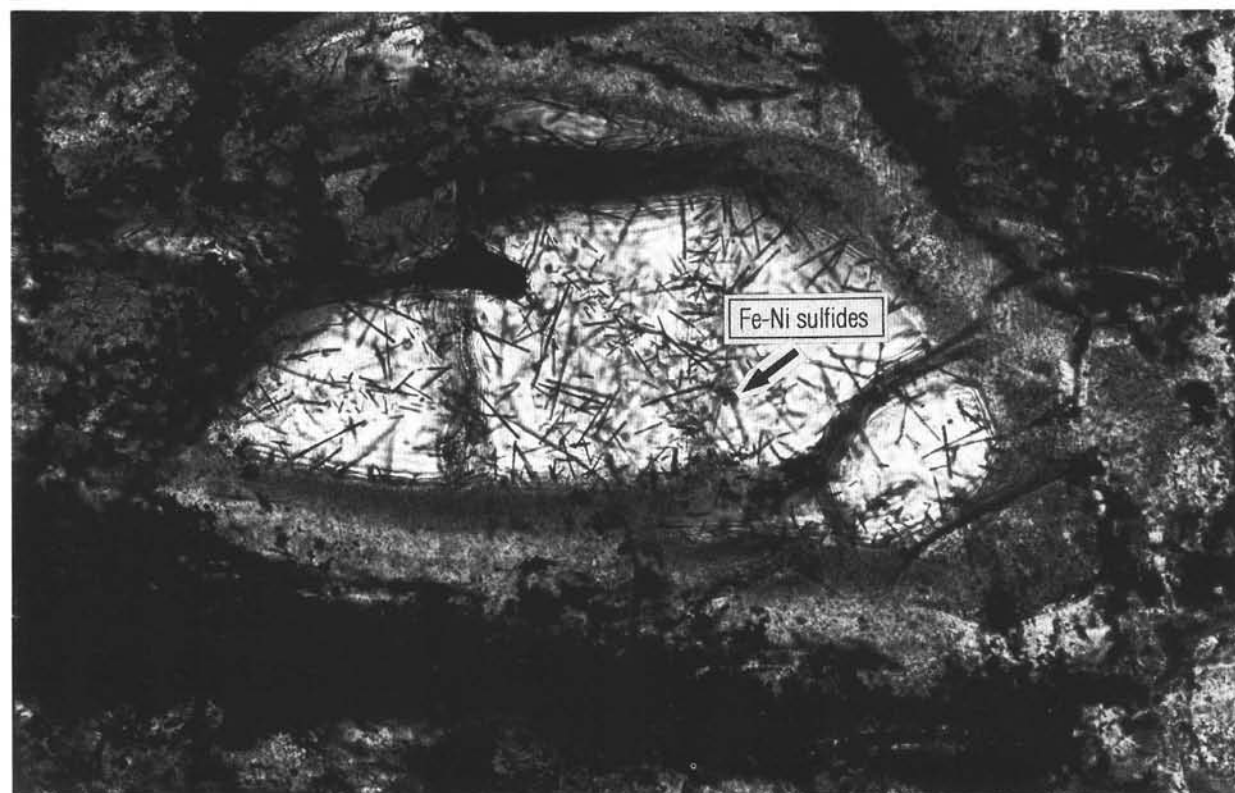
Figure 3. Photomicrographs of serpentinization textures in the peridotites from Holes 920B and 920D. A. Mesh texture serpentine + brucite. Mesh rim is composed of lizardite (colorless), whereas mesh center (dark) is composed of finely intergrown serpentine + brucite. Fibrous chrysotile extension vein follows the margins of mesh cell. Sp + bru = mesh textured serpentine + brucite. Plane-polarized light. Field of view is 2 mm long. Sample 153-920B-12R-2, 143–147 cm. B. Acicular Fe-Ni sulfides within mesh texture. Sulfides occur within mesh center serpentine. Plane-polarized light. Field of view is 1 mm long. Sample 153-920B-1W-1, 91–98 cm.
