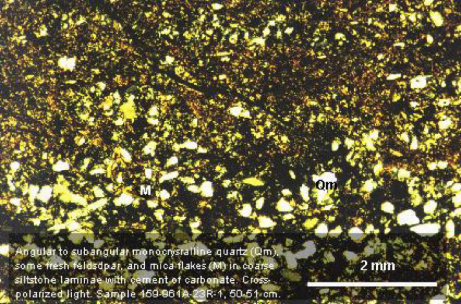
Angular to subangular monocrystalline quartz (Qm), some fresh feldspar, and mica flakes (M) in coarse siltstone laminae with cement of carbonate. Cross-polarized light. Sample 159-961A-23R-1, 50.51 cm.
