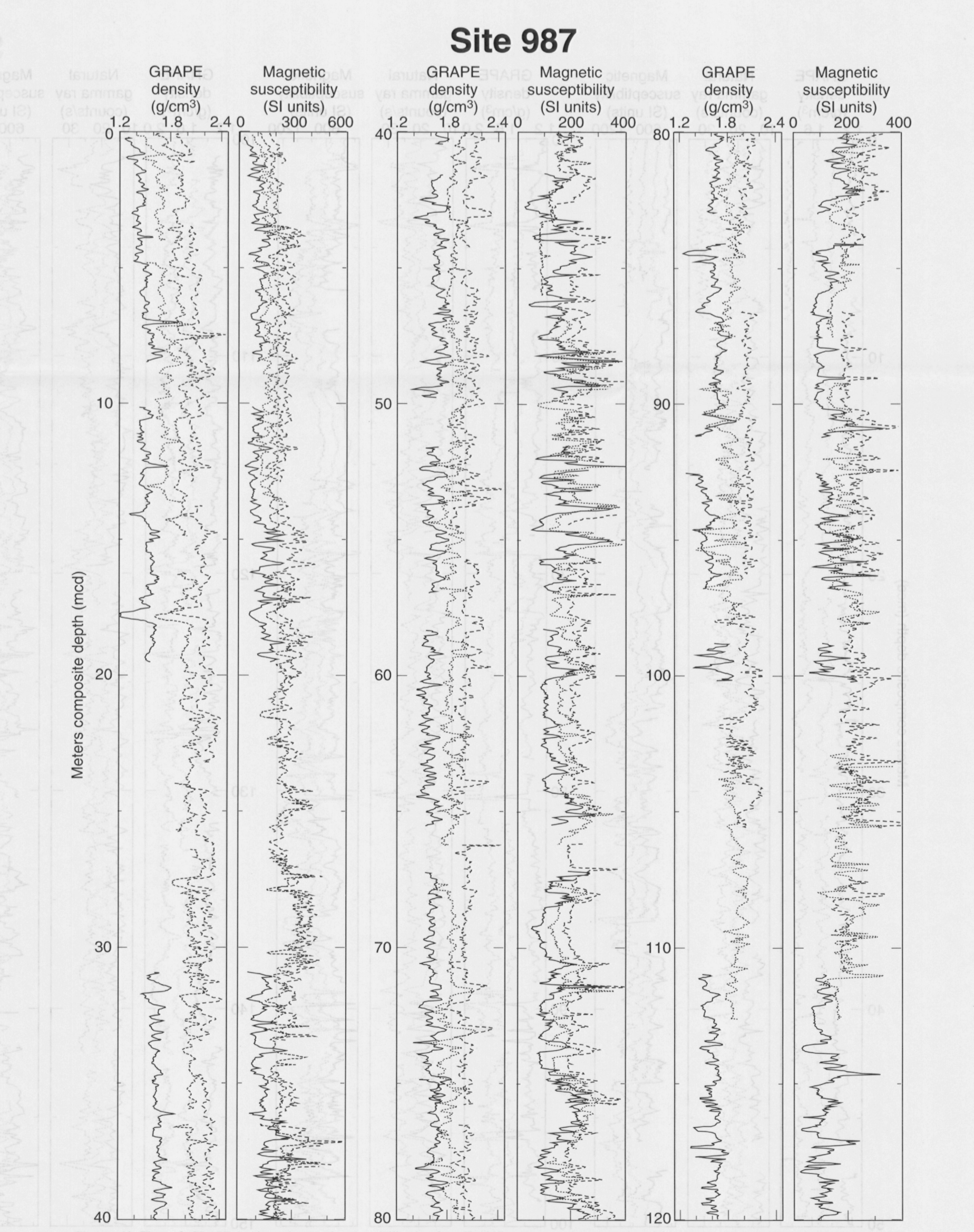
Chapter 10: Figure 2. GRAPE density and magnetic susceptibility data from Site 987 on the mcd (meters composite depth) scale. Lines for Holes 987B (dotted), 987C (dashed), and 987D (long dashed) have been horizontally offset from line for Hole 987A (solid) for better display; therefore, values given on horizontal scale are the true values only for Hole 987A.
