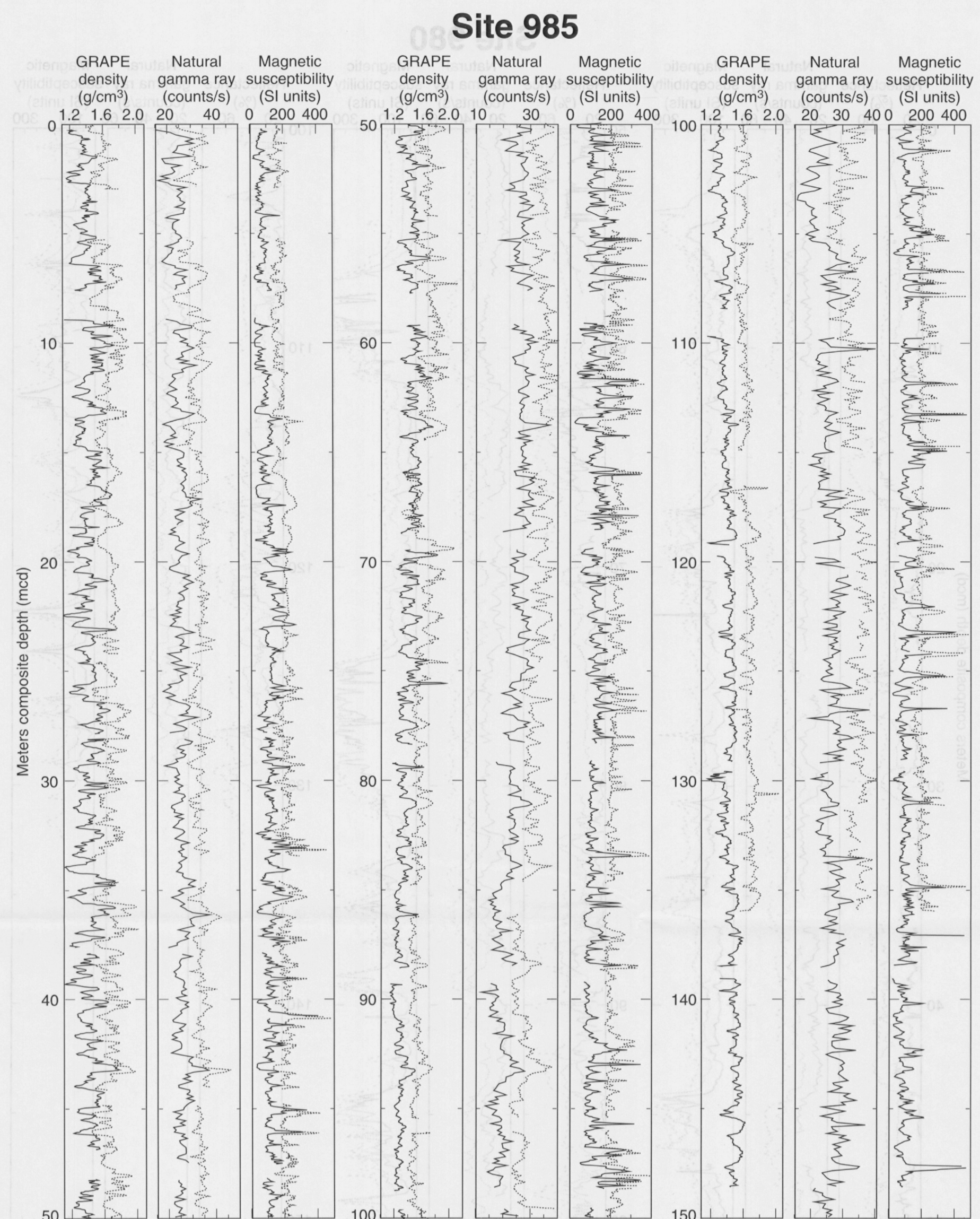
Chapter 8: Figure 3. GRAPE density, natural gamma radiation, and magnetic susceptibility data from Site 985 on the mcd (meters composite depth) scale. Line for Hole 985B (dotted) has been horizontally offset from line for Hole 985A (solid) for better display; therefore, values given on horizontal scale are the true values only for Hole 985A.
