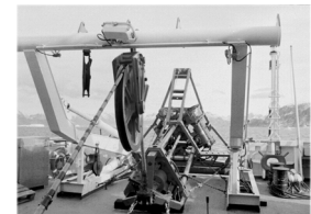
F3. Secured Rockdrill, p. 7.
