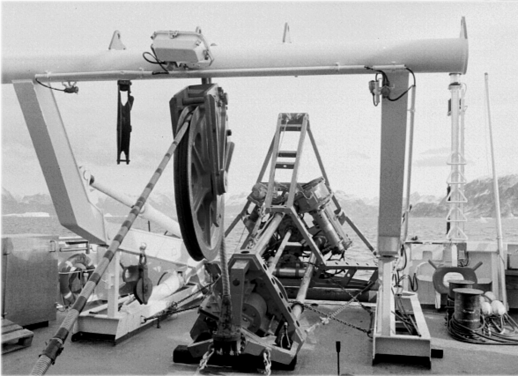
Figure F3. British Geological Survey–modified 3-m Rockdrill secured during transit on the aft deck of Aranda in 1999. The East Greenland coast of uplifted Precambrian basement is visible in the background.
