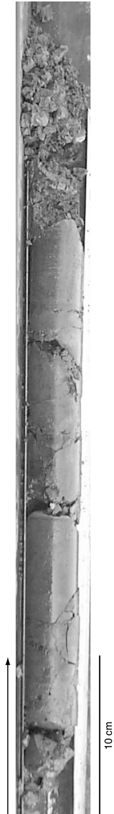
Figure F2. Highly fractured basalt recovered by wireline diamond coring system on the Norskald (Piece SEG02A-5-1, 20–55 cm). Core diameter is 56 mm. Arrow on the left indicates stratigraphic up direction.
