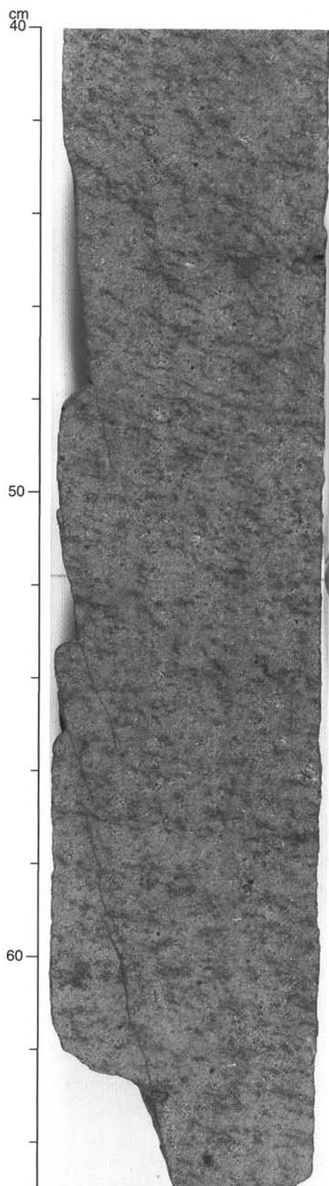
Figure 11. Photograph of Section 163-990A-14R-2 (Piece 5A, 40–65 cm) showing steeply dipping en echelon fractures related to subvertical brittle shearing of the basalts.
