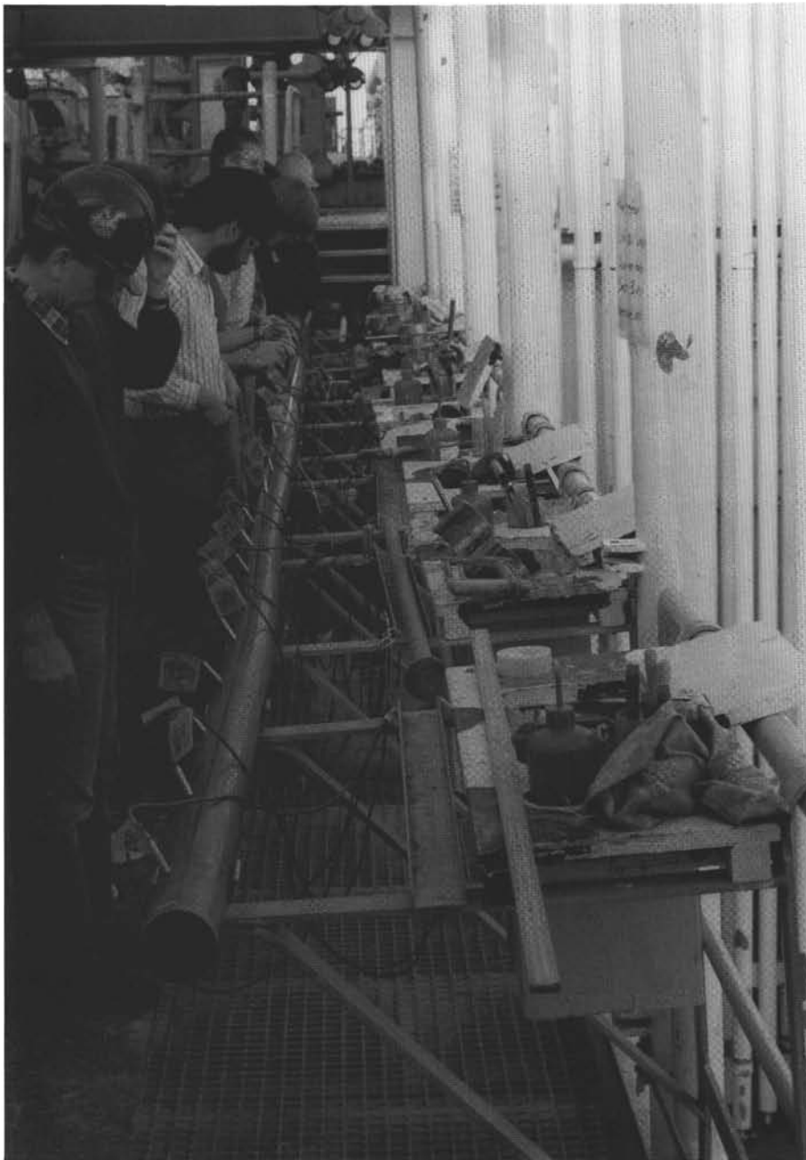
Photograph illustrating core temperature measurements being made on the catwalk of the JOIDES Resolution during Leg 164. Thirty thermocouple probes are inserted into the core through small holes in the core liner as the data are logged on a personal computer. Temperature measurements are useful for detecting gas hydrate because gas hydrate decomposition is endothermic. Thus, anomalously low temperatures may indicate areas where gas hydrate is decomposing or has decomposed.
