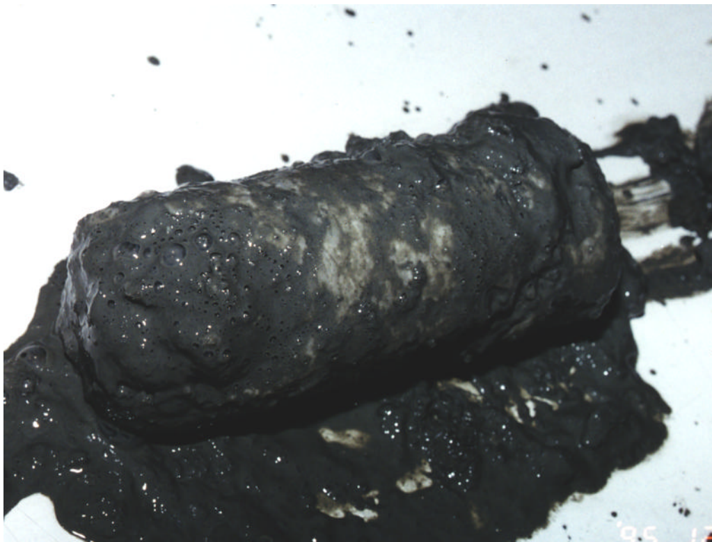
Figure 2. Photograph of a nearly pure piece of gas hydrate that is ~5 cm × 14 cm in size and coated by a thin veneer of a mud-rich slurry that presumably formed from the adjacent greenish gray nannofossil-rich clay (Section 164-997A-42X-3; 331 mbsf). Note the bubbles within the slurry.
