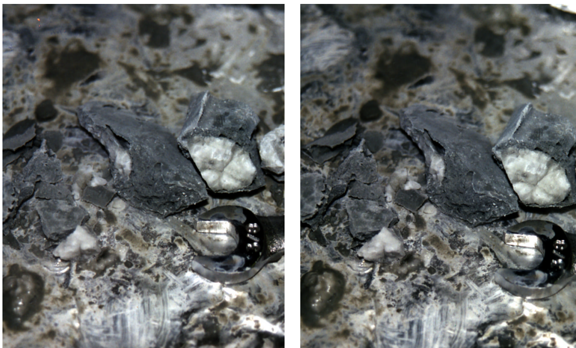
Figure 4. Stereophotographic pair showing freshly broken face of a white gas hydrate nodule hosted inside gray carbonate cemented crust (Section 164-996B-1H-3; 2.2 mbsf). The \frac{3}{8} -in (0.95 cm) wrench is for scale.
