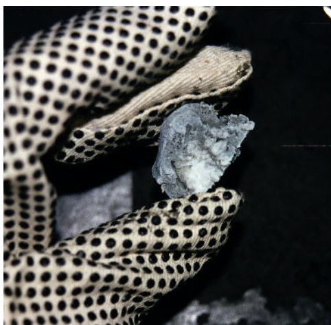
Figure 8. The face of a freshly broken nodule with a gas hydrate-filled core (Section 164-996B-1H-2; 1.92 mbsf). Note that the gas hydrate is cut by thin sediment-filled veins. The gloved hand is for scale.
