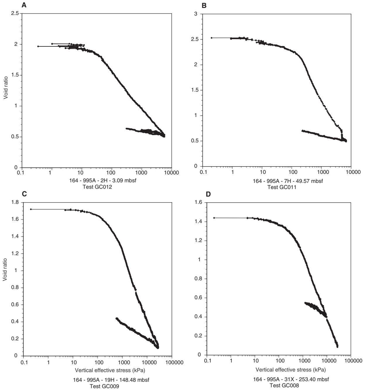
Figure 4. A–H. Consolidation test results from Hole 995A. (Continued next page.)
