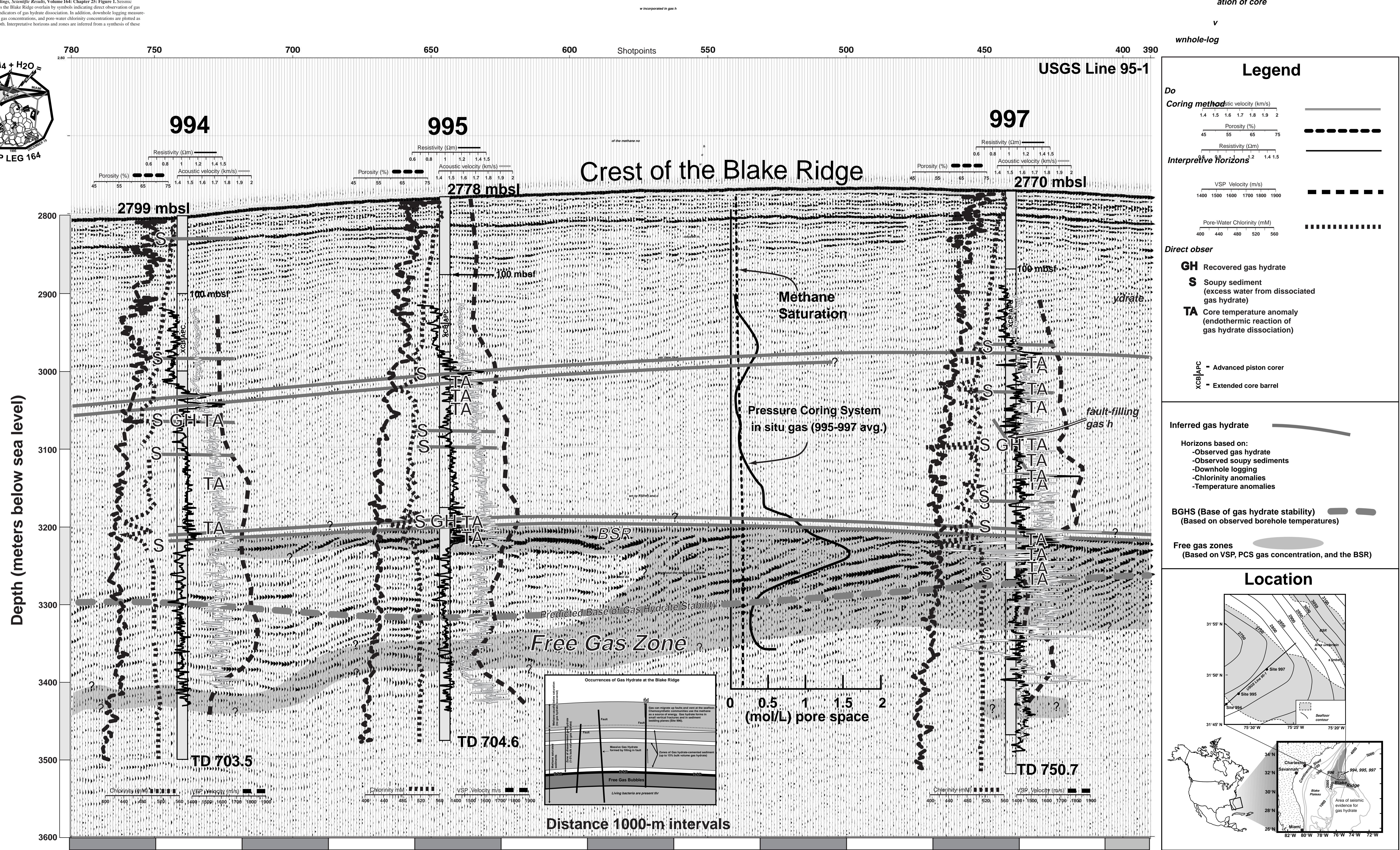
**ODP Proceedings, Scientific Results, Volume 164: Chapter 25: Figure 1.** Seismic transect across the Blake Ridge overlain by symbols indicating direct observation of gas hydrate and indicators of gas hydrate dissociation. In addition, downhole logging measurements, in situ gas concentrations, and pore-water chlorinity concentrations are plotted as lines with depth. Interpretative horizons and zones are inferred from a synthesis of these observations.
