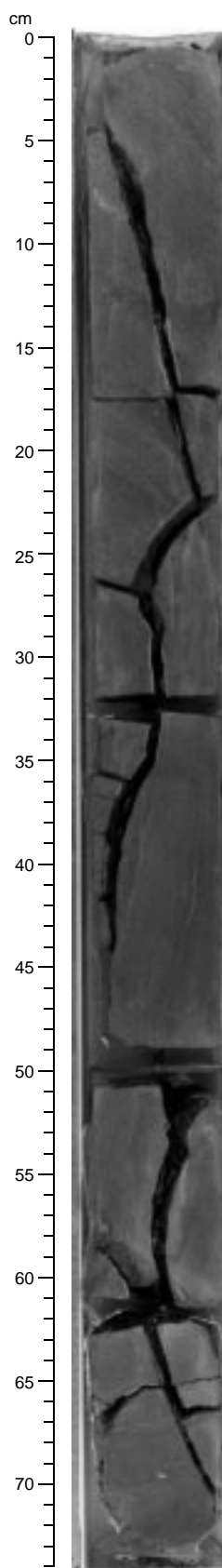
Figure 15. Close-up photograph of the diabasic sill grading down to the aphanitic chilled basaltic margin at the base (interval 168-1027C-1R-6, 0–74 cm). The core is cut by an anastomosing fracture lined by secondary carbonate and clay.
