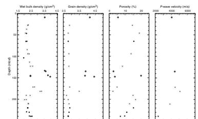
F4. Shore-based and shipboard index properties data plots, Hole 856H, p. 13.
