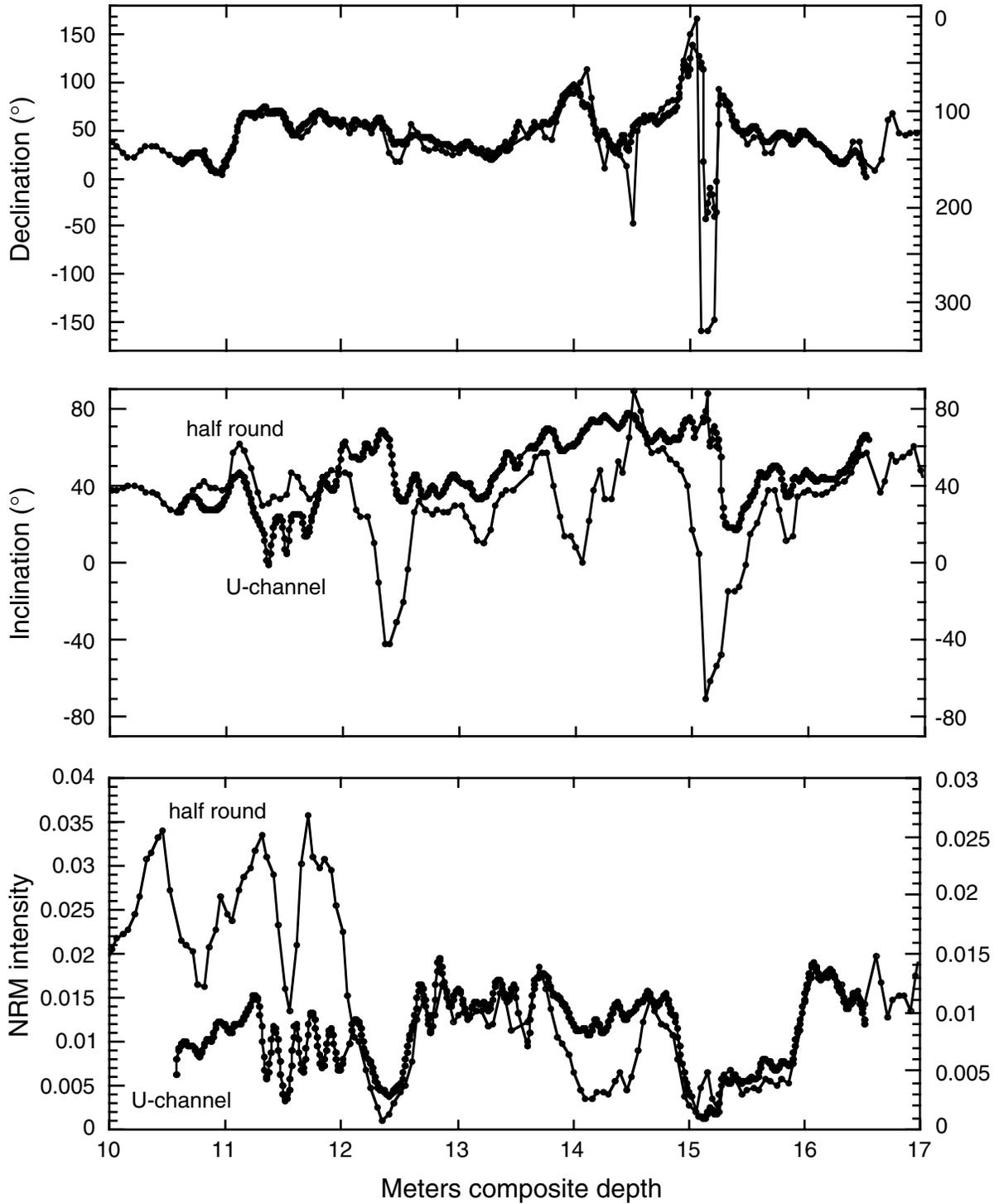
Figure F6. Comparison of shipboard (half round) and U-channel long-core paleomagnetic measurements (after 20-mT AF demagnetization) for an interval containing excursions  $3\alpha$  and  $3\beta$  in Hole 1061C. See “U-Channel Paleomagnetic Measurements of Excursions  $3\alpha$  and  $3\beta$ ,” p. 3, for more detailed discussion.
