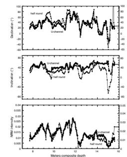
F7. Comparison of half-round and U-channel long-core paleomagnetic measurements, Hole 1063C, p. 17.
