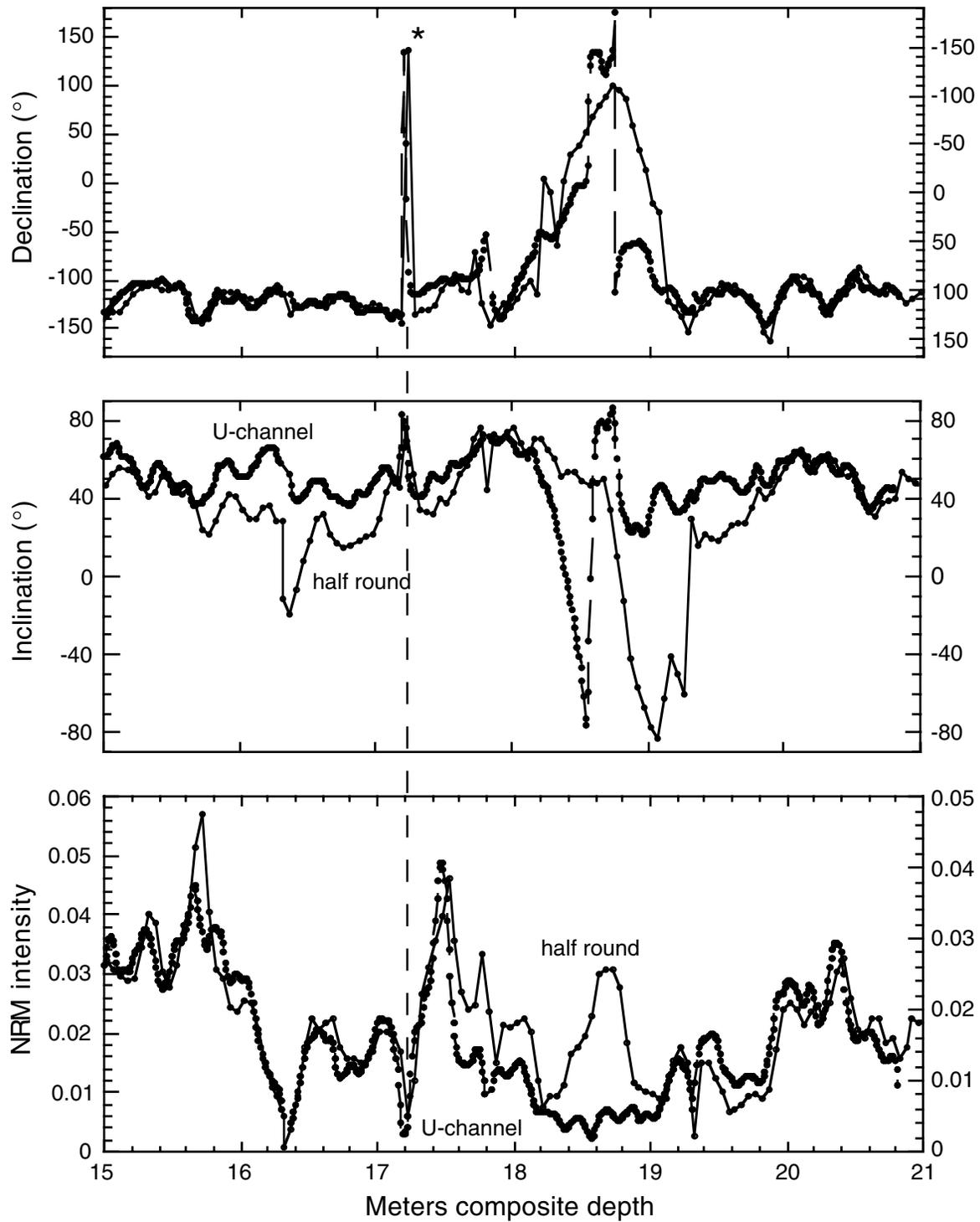
Figure F8. A comparison of excursion  $3\beta$  as recorded in Holes 1061B and 1061C. The depth scale is provided by magnetic susceptibility correlations between all the holes at Site 1061. There are still ~20 cm offsets between equivalent individual paleomagnetic features at the two holes due to more subtle variations in sediment accumulation at the two holes.
