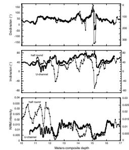
F6. Comparison of half-round and U-channel long-core paleomagnetic measurements, Hole 1061C, p. 16.
