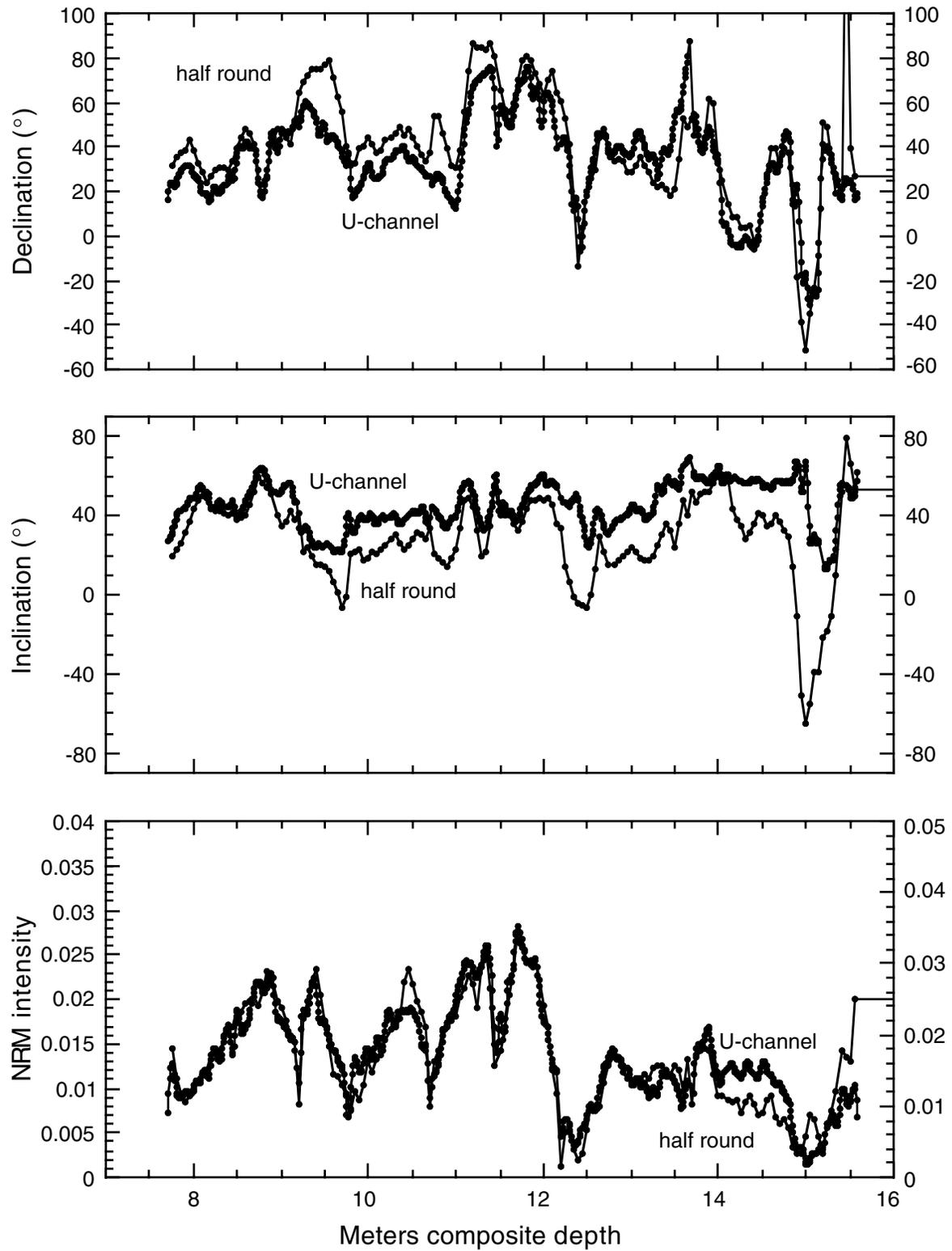
Figure F7. Comparison of shipboard (half round) and U-channel long-core paleomagnetic measurements (after 20 -mT AF demagnetization) for an interval containing excursions 3 $\alpha$  and 3 $\beta$  in Hole 1063C. See "U-Channel Paleomagnetic Measurements of Excursions 3 $\alpha$  and 3 $\beta$ ," p. 3, for more detailed discussion.
