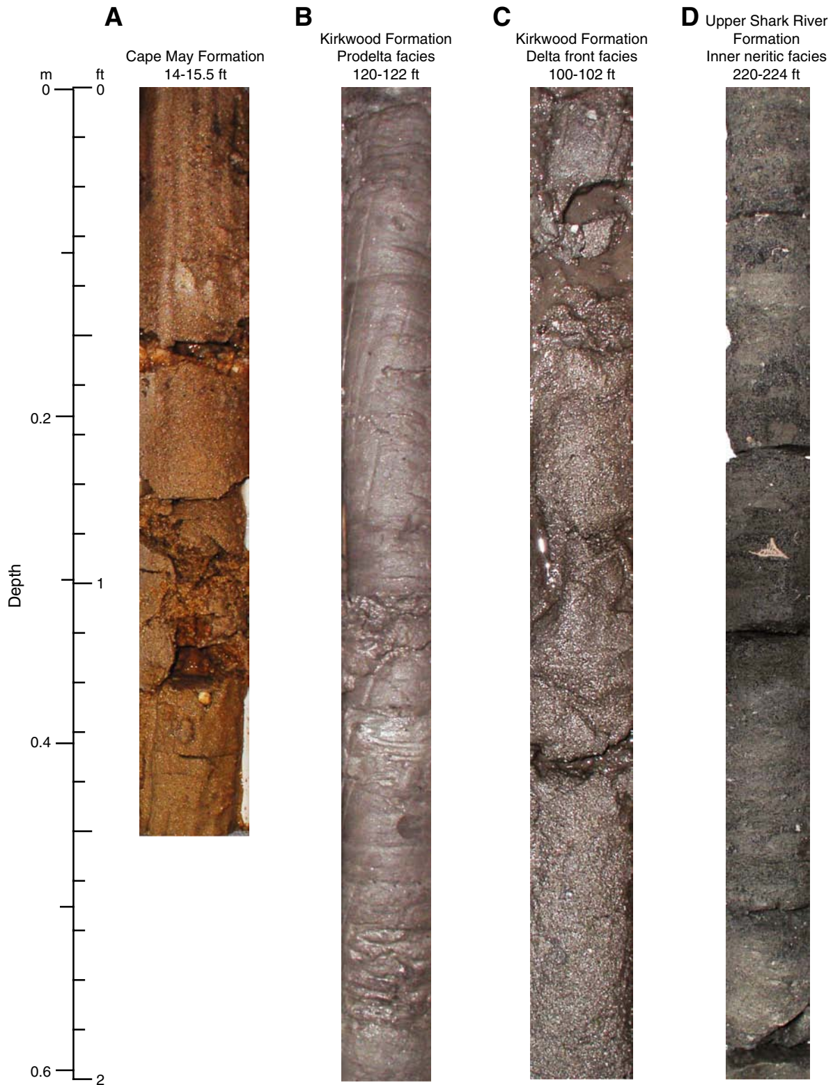
Figure F10. A. Medium sand from the Cape May Formation (14–15.5 ft; 4.27–4.72 m). B. Silty clay representing a prodelta environment from the Kirkwood Formation (120–122 ft; 36.58–37.19 m). C. Sand representing a delta front environment from the Kirkwood Formation (100–102 ft; 30.48–31.09 m). D. Inner neritic sand from the upper Shark River Formation (220–224 ft; 67.06–68.8 m).
