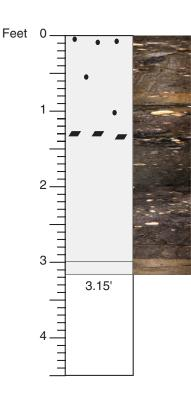
SAND: medium to coarse; abundant pebbles up to 4 cm and granules; abundant lignite at 1.3-1.4 ft, harder brown clay layer at plastic sheet, above is fill, below is probably good core, fewer pebbles down core; very dark gray (10YR 3/1)
