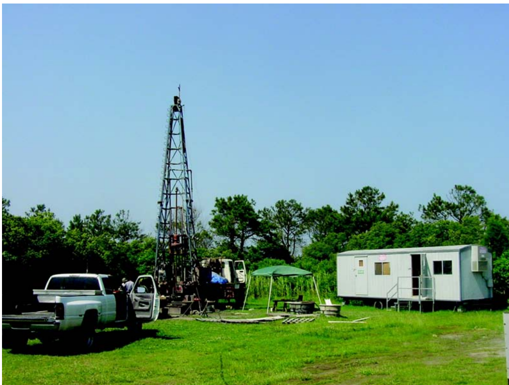
Frontispiece 3. Bethany Beach Site. U.S. Geological Survey, Eastern Earth Surface Processes Team truck-mounted drill rig at the Bethany Beach, Delaware, drill site (May–June 2000). The trailer on the right was used as a field laboratory.
