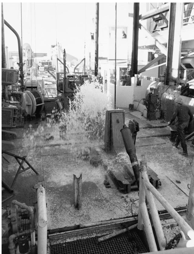
Figure 25. A fountain of water gushing from the drill pipe at the rig floor at Site 1071. Initial fountain height was estimated at half the height of the derrick (~30 m). Note the significant quantity of sand deposited on the rig floor by the fountain.
