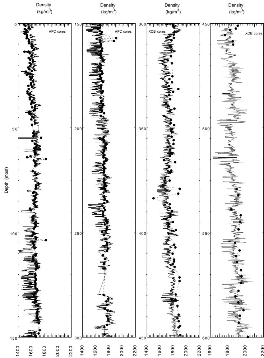
Figure 31. GRAPE wet bulk density data (solid lines) compared with discrete gravimetric wet bulk density values (solid circles) for Hole 1085A.
