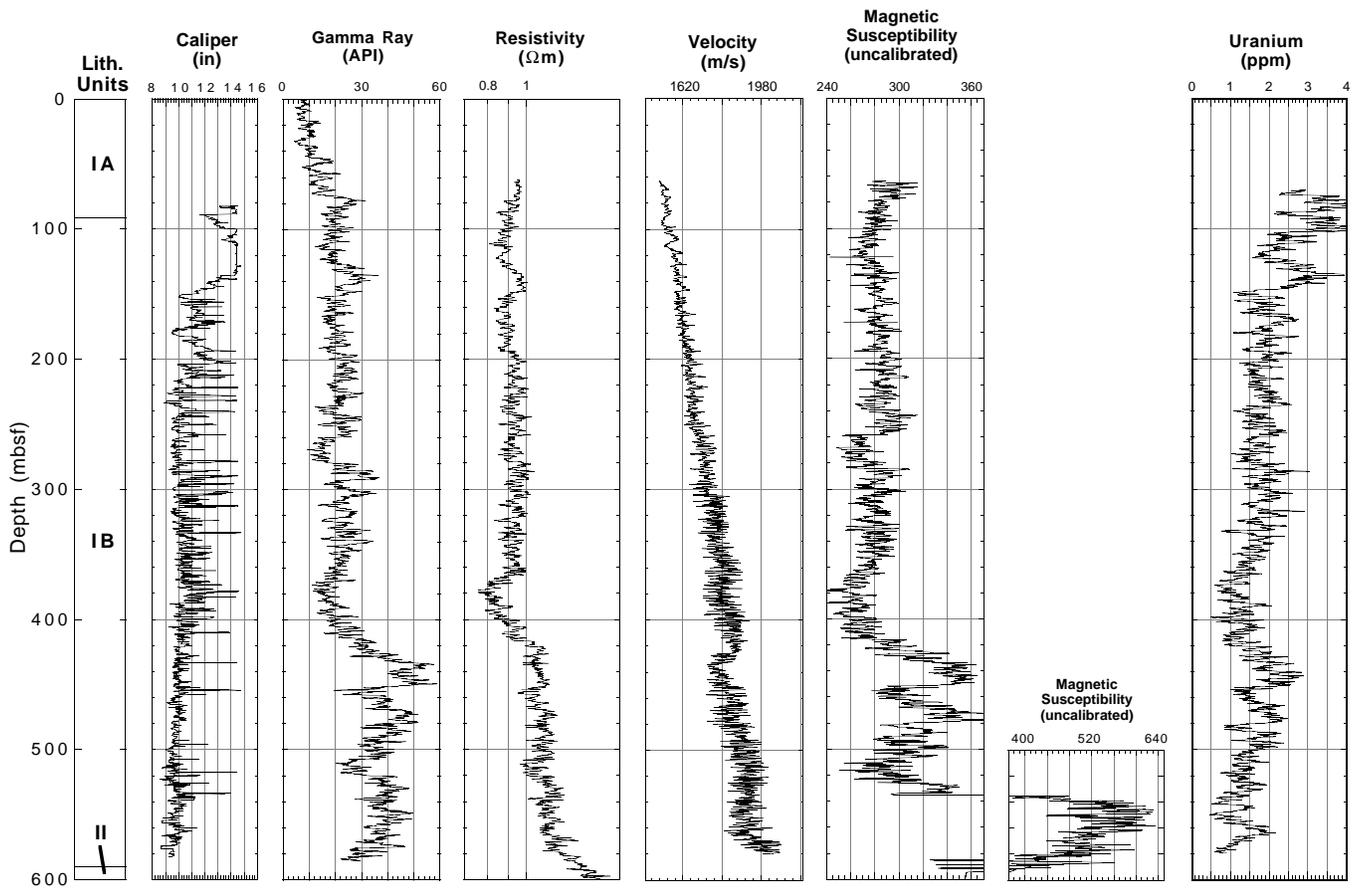
Figure 36. Downhole logs of caliper, natural gamma-ray, resistivity, velocity, magnetic susceptibility, and uranium content for Hole 1085A.
