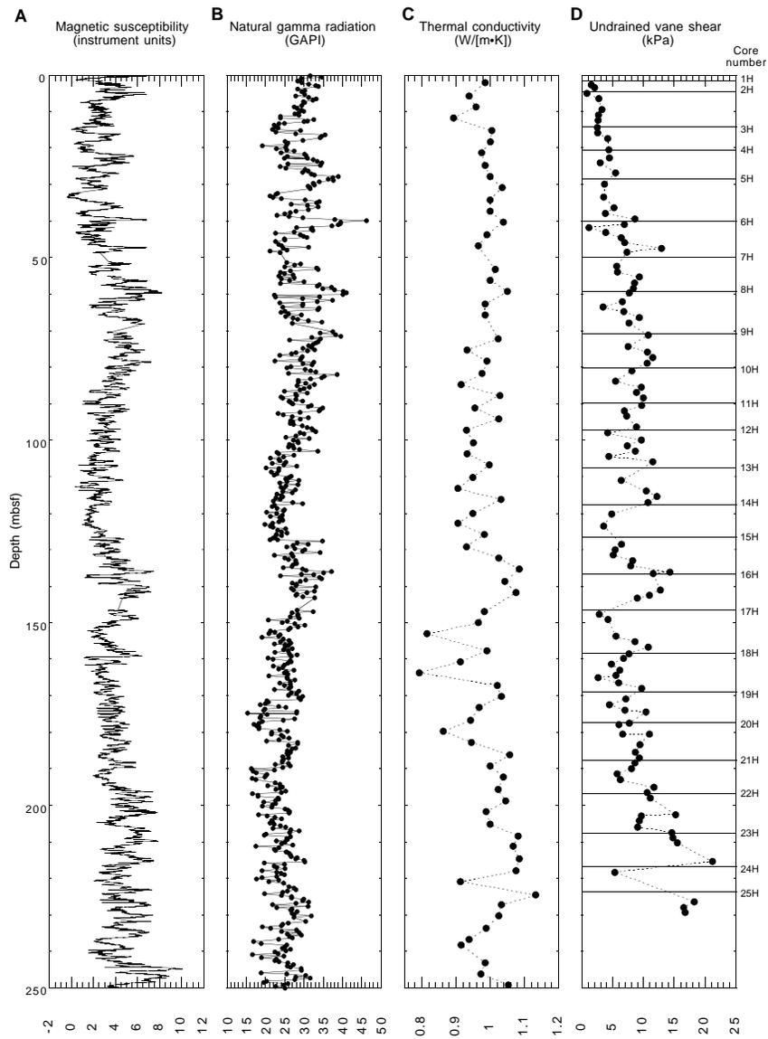
Figure 33. Plots of (A) magnetic susceptibility and (B) natural gamma radiation from MST measurements compared with discrete values of (C) thermal conductivity and (D) undrained vane shear strength between 0 and 250 mbsf for Hole 1085A.
