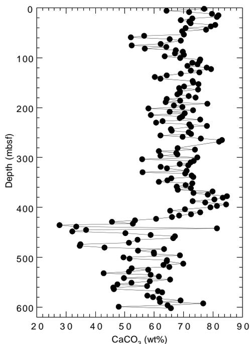
Figure 24. Concentrations of CaCO<sub>3</sub> in sediments from Hole 1085A. Variations reflect light-dark color cycles and different lithologic units.
