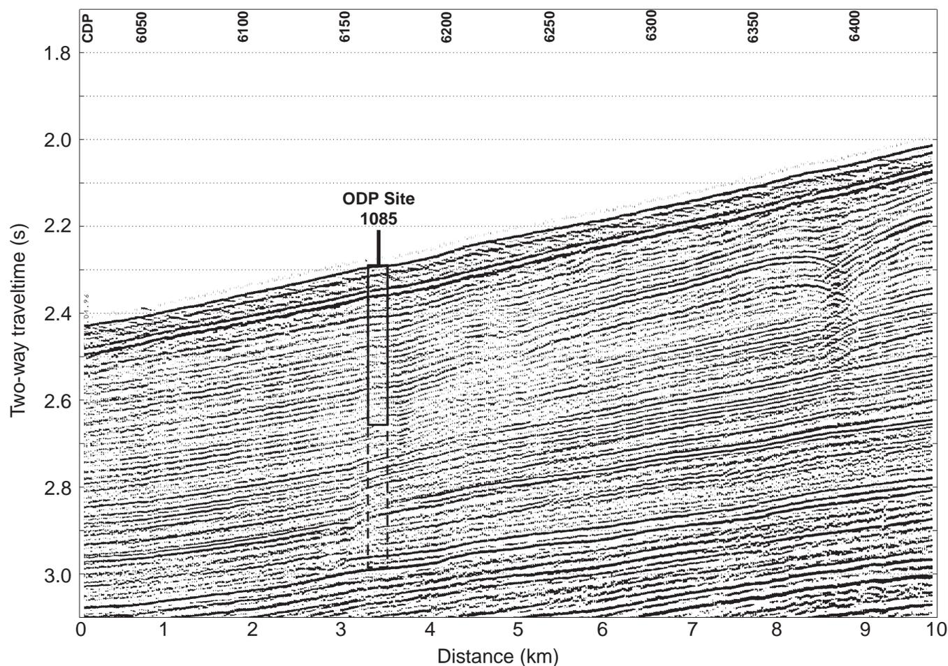
Figure 3. Seismic section of Line GeoB/AWI 96-009 at Site 1085. Vertical axis is given in TWT. CDP interval is 25 m for a shotpoint spacing of 25 m. Site 1085 is located at CDP 6163. The box indicates the approximate penetration of the borehole of 300 m (APC) and 600 m (XCB), respectively.
