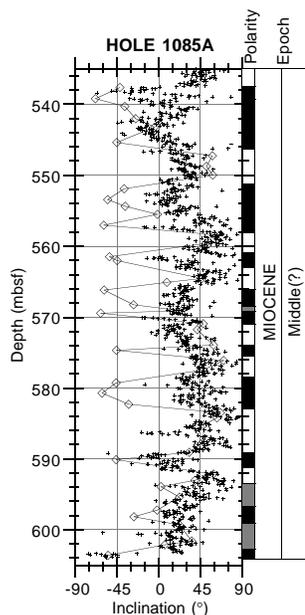
Figure 15. Inclination data and magnetostratigraphic interpretation, after 20-mT demagnetization, from half-core measurements and discrete samples from 535 to 605 mbsf at Hole 1085A. Black symbols = half-core measurements with no Tensor correction; open diamonds = discrete samples. Polarity shading: black = normal, white = reversed, and gray = ambiguous.
