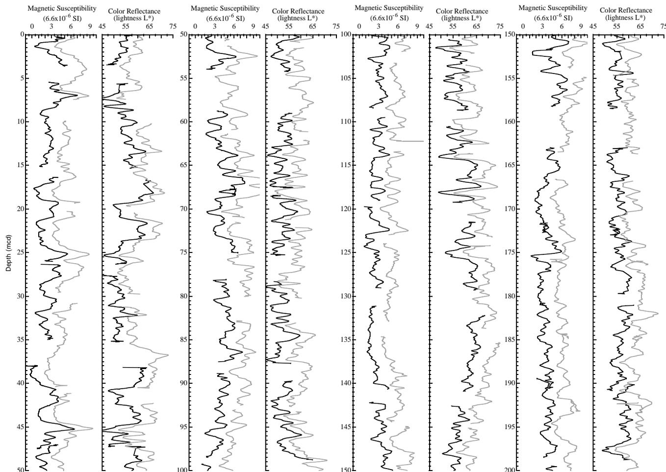
Figure 16. Composite section for Site 1085. Magnetic susceptibility and total color reflectance (lightness L\*) are plotted for Holes 1085A (black line) and 1085B (gray line). The downhole logs are shown in meters composite depth (mcd). Offsets have been applied for clarity. (Continued next page.)
