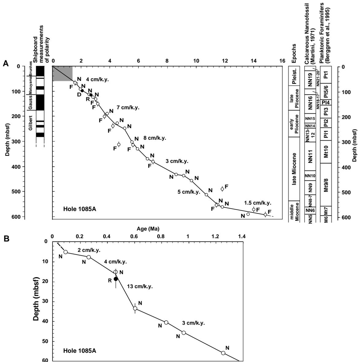
Figure 12. Age-depth plot and sedimentation rates estimated from calcareous microfossil (open circles; F = planktonic foraminifers and N = calcareous nannofossils) and siliceous microfossil (closed circles; D = diatoms and R = radiolarians) datums at Hole 1085A. Data are shown for (A) the Miocene and Pliocene of Hole 1085A and (B) the last 1.4 m.y. of Hole 1085A.
