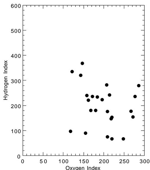
Figure 27. Rock-Eval Van Krevelen-type diagram of sediments from Hole 1085A. Organic matter appears to be type II algal material that has been variably oxidized. HI = milligrams of hydrocarbons per gram of organic carbon; OI = milligrams of CO<sub>2</sub> per gram of organic carbon.
