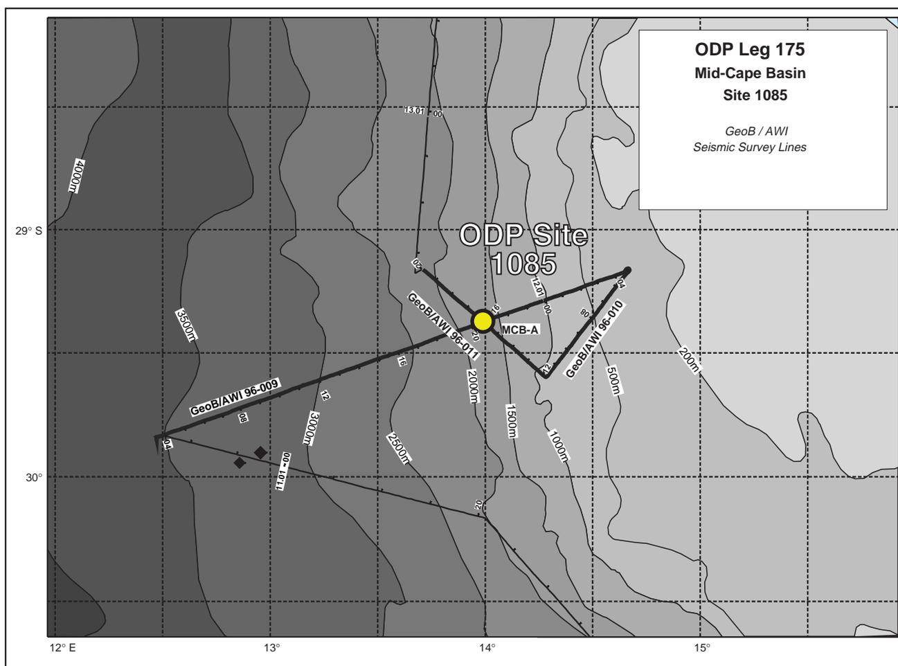
Figure 2. Map of seismic presite survey lines, proposed site locations, and ODP Leg 175 drill Site 1085 in the Mid-Cape Basin. Bathymetry was derived from Gebco Digital Dataset on CD-ROM.
