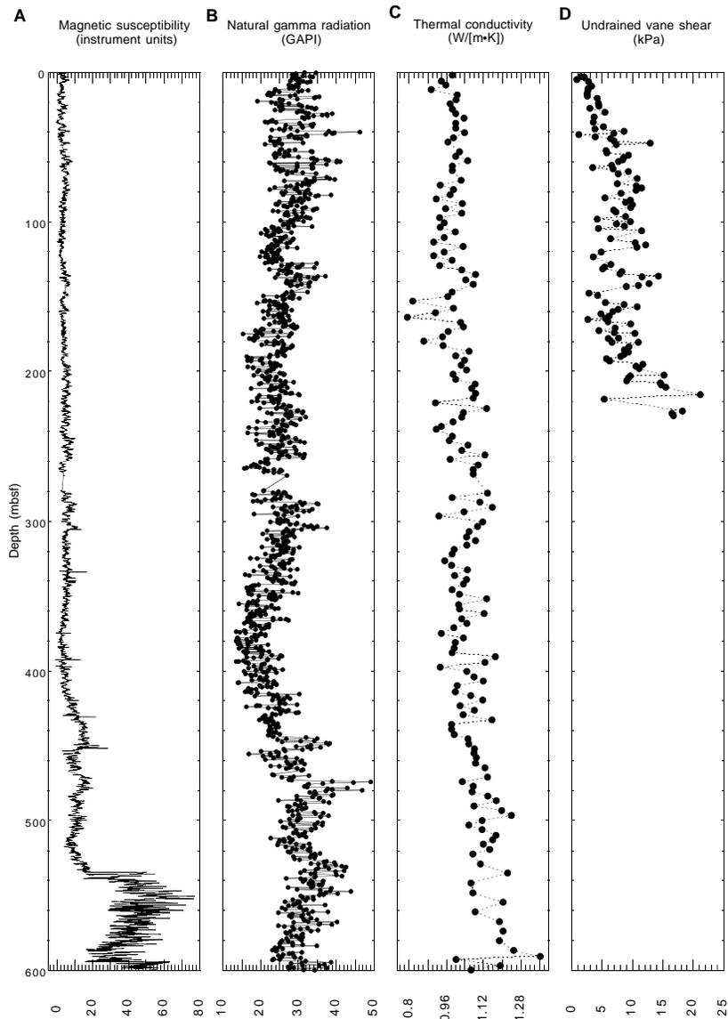
Figure 34. Plots of (A) magnetic susceptibility and (B) natural gamma radiation from MST measurements compared with discrete values of (C) thermal conductivity and (D) undrained vane shear strength between 0 and 600 mbsf for Hole 1085A.
