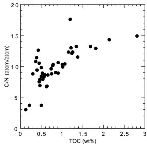
Figure 26. Comparison of organic matter C/N ratios and TOC concentrations of sediments from Hole 1085A. The correspondence between increases in both parameters indicates that preservation of marine organic matter during early diagenesis is important to enhancing the organic carbon richness of sediments on the Walvis Ridge.
