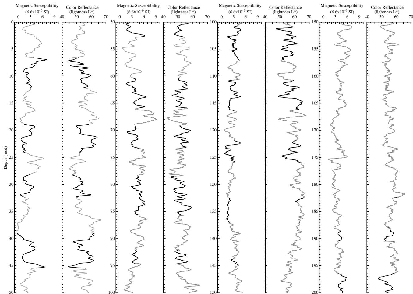
Figure 17. The spliced records for magnetic susceptibility and total color reflectance (lightness  $L^*$ ) are plotted in meters composite depth (mcd). Cores from Holes 1085A and 1085B have been used for the spliced record: black line = Hole 1085A and gray line = Hole 1085B. (Continued next page.)
