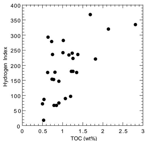
Figure 28. Comparison of Rock-Eval HI values and TOC concentrations of sediments from Hole 1085A. The correspondence between increases in both parameters indicates that preservation of marine organic matter is important to enhancing the organic carbon richness of sediments on the Walvis Ridge.
