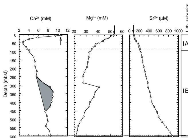
Figure 20. Downcore profiles of Ca<sup>2+</sup>, Mg<sup>2+</sup>, and Sr<sup>2+</sup> at Site 1085. Lithostratigraphic subunits shown on right-hand bar, with Unit II too small to indicate. Shaded region = depth interval of elevated dissolved Ca<sup>2+</sup> concentrations. Arrows = mean ocean-bottom-water values taken from Millero and Sohn (1992).
