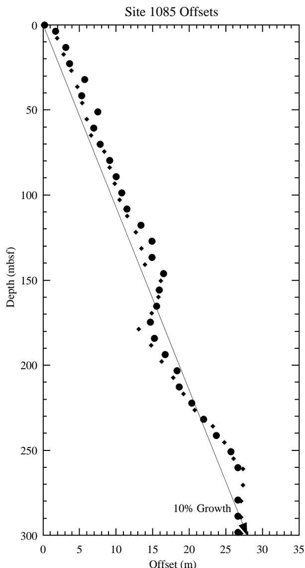
Figure 18. Cores offsets applied to Site 1085 plotted against standard ODP meters below seafloor (mbsf). A linear 10% growth of meters composite depth (mcd) compared with mbsf is indicated by an arrow. Offsets are plotted for Holes 1085A (circles) and 1085B (diamonds).
