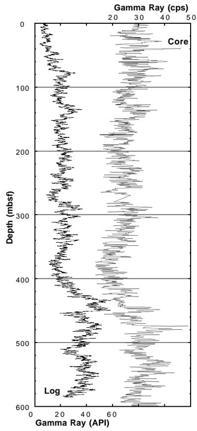
Figure 37. Comparison of core (MST) and log natural gamma-ray data for Hole 1085A.
