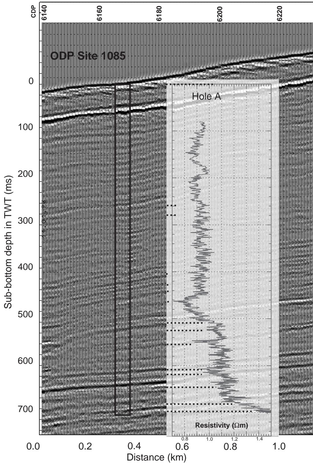
Figure 4. Close-up of Line GeoB/AWI 96-009 near Site 1085. Vertical axis is given in TWT. Amplitudes are grayscale. For comparison, the resistivity log from downhole logging is shown. Logging depth is transferred to TWT using the logging results. Selected reflectors can be correlated with local extremes in the resistivity log (straight thick dashed lines).
