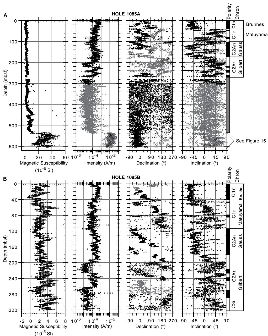
Figure 14. Magnetic susceptibility (SI volume units) and NRM intensity, declination, inclination, and magnetostratigraphic interpretation after 20-mT demagnetization for (A) Hole 1085A and (B) Hole 1085B. Black symbols = Tensor corrected; gray symbols = uncorrected; open diamonds = discrete samples. Polarity shading: black = normal, white = reversed, and gray = ambiguous.
