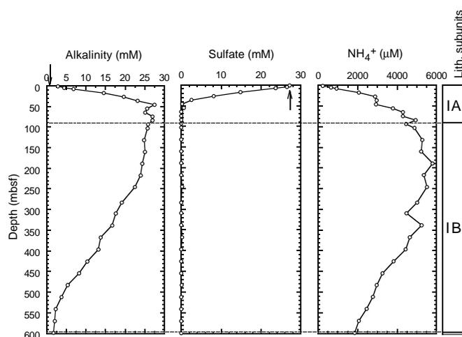
Figure 19. Downcore profiles of dissolved alkalinity, sulfate, and ammonium at Site 1085. Lithostratigraphic subunits shown on right-hand bar, with Unit II too small to indicate. Arrows = mean ocean-bottom-water values taken from Millero and Sohn (1992).
