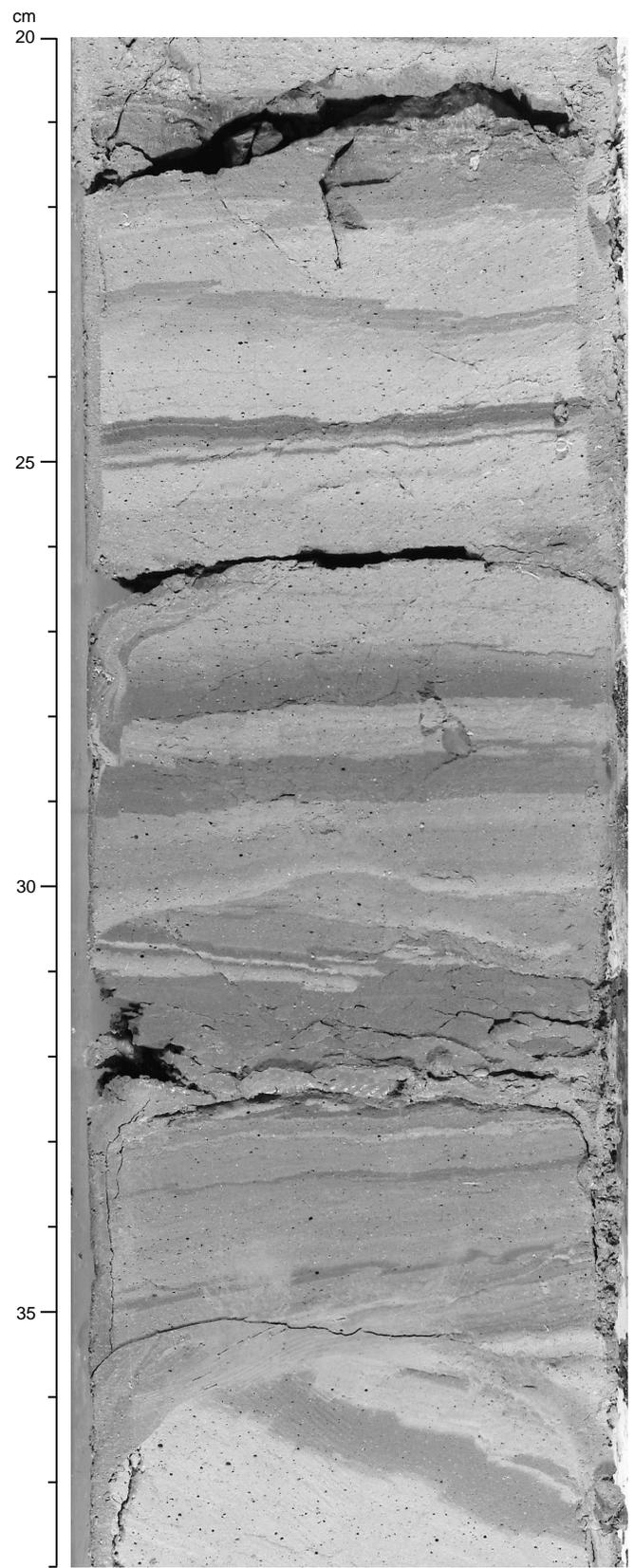
Figure 8. Microfaulting of reddish brown, clay-rich nanofossil ooze in the core catcher of Core 175-1085A-63X.
