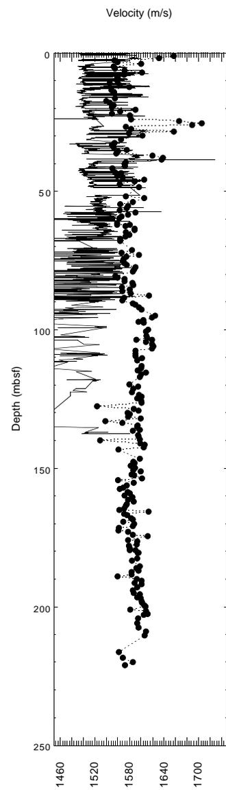
Figure 32. Discrete velocity profile (solid circles) compared with MST velocity data (solid line) measured at Hole 1085A.
