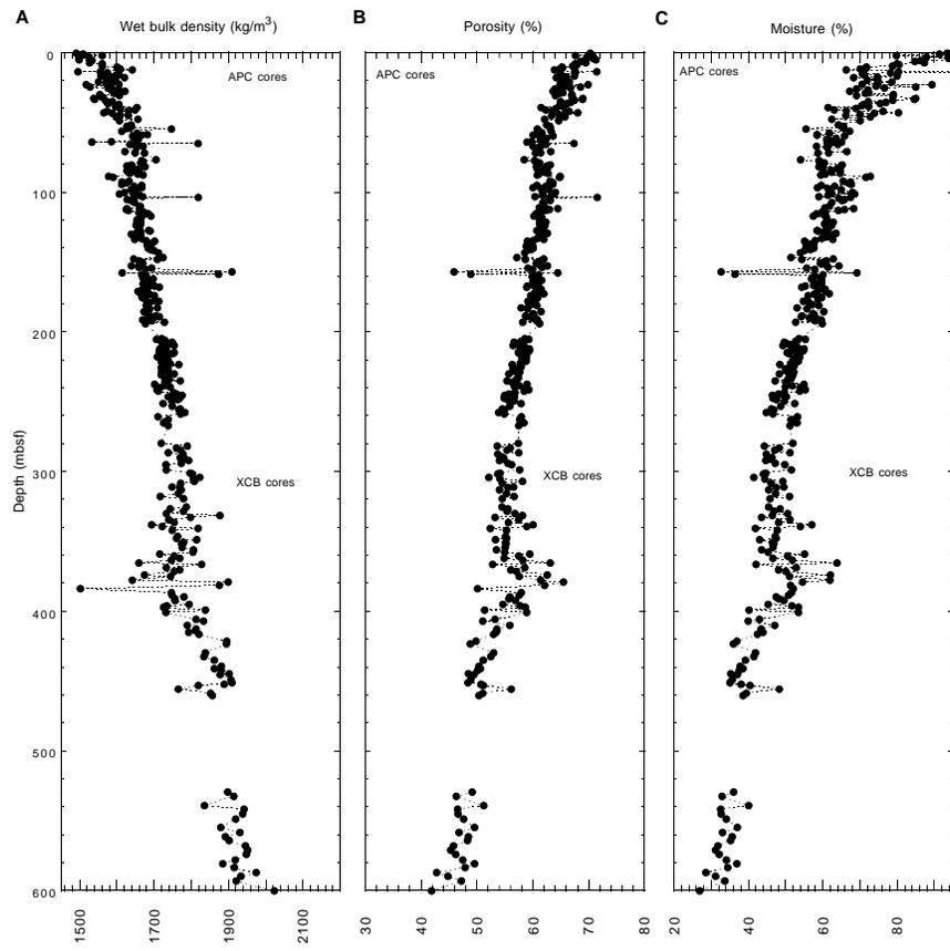
Figure 35. Gravimetric (A) wet bulk density, (B) porosity, and (C) moisture content derived from index properties measurements at Hole 1085A.
