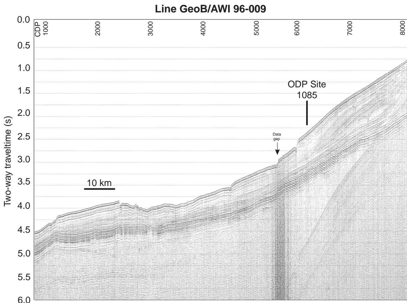
Figure 1. Seismic Line GeoB/AWI 96-009 with Site 1085. Vertical axis is given in TWT. CDP interval is 25 m for a shotpoint spacing of 25 m. Seismic data is 24-fold stacked and not migrated. Site 1085 is located at CDP 6163.
