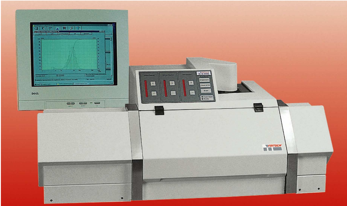
Figure F4. A. Layout of the laser particle sizer “Analysette 22”-Economy (Fritsch GmbH Laborgerätebau, 1994). The unit is equipped with a 632.8-nm wavelength and 3-mW helium-neon laser and handles suspensions with a particle size between 0.1 and 600 \mu\text{m} . B, C. The unique fixed focus size analyzing system with particle size range-dependent cell shift. Shifting the sampling cell relative to the detector changes the diffraction angle and the size of the sensor area affected. A large distance between sampling cell and detector therefore permits the measurement of larger particles with a smaller diffraction angle, and short distances are used for small particles with a wide diffraction angle.
